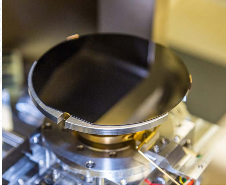
Original nanopikes grown on silicon wafers
