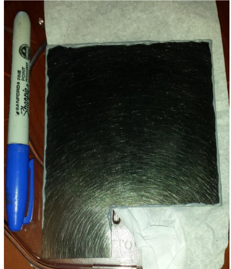
Successfully growing nanopikes on metallic substrates
