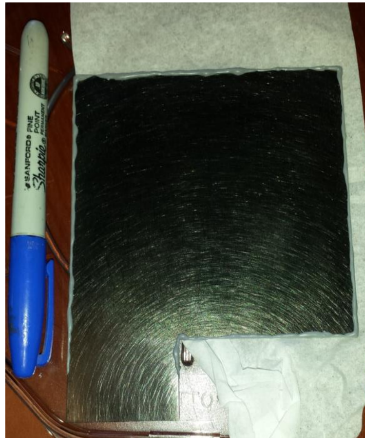
Successfully growing nanospikes on metallic substrates
