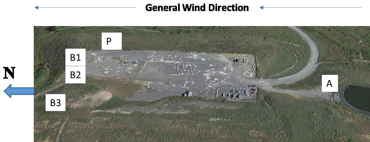
Figure 5.2: General layout of indirect methane monitoring during Audit 6.
