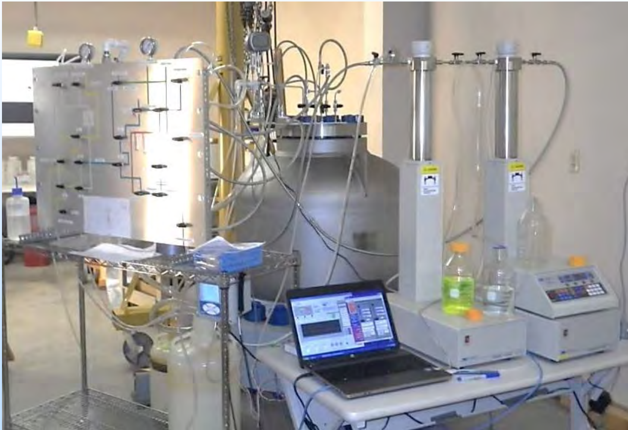
Phillips, AJ, Eldring, J, Hiebert, R, Lauchnor, E, Mitchell, AC, Gerlach, R, Cunningham, A, and Spangler, L. High pressure test vessel for the examination of biogeochemical processes. J. Petrol. Sci. Eng. 126, February 2015:55-62, DOI: 10.1016/j.petrol.2014.12.008
