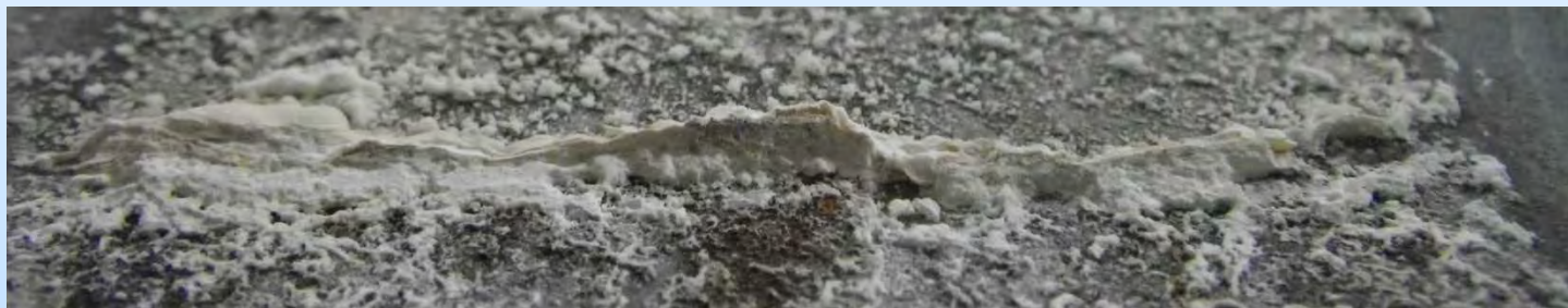
Carbonate seal on cement side of the fracture fixture formed right at the interface of the 0.2mm gap
