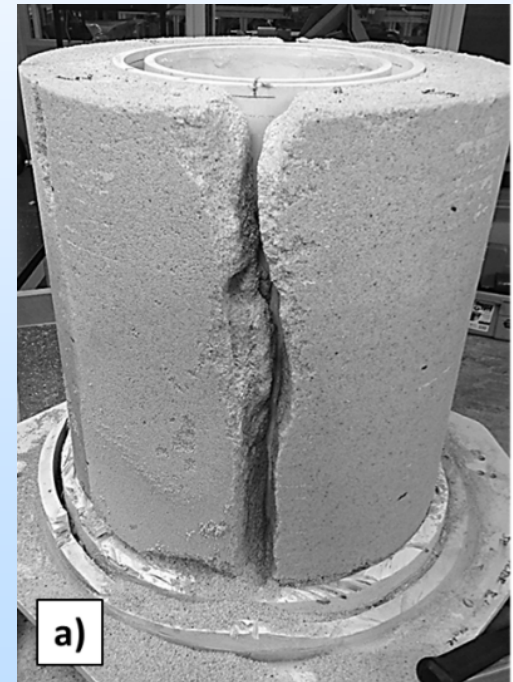
Figure 3. The biomineralized sand annulus was destructively sampled to quantify calcite precipitation. The outer pipes of the bioreactor were cut away to expose the biomineralized sand annulus. A saw was used to cut the annulus into quarters, producing the large crack shown here.
