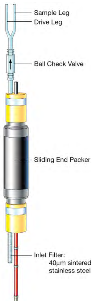
Figure 10.4—Schematic of the U-tube sampling device (source: JGR, Freifeld et al, 2005).
