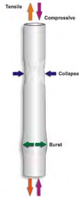
Figure 8.3—Schematic of stresses on the well bore (source; USEPA, 2012b).
