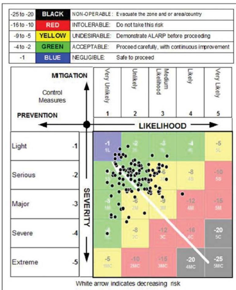
Figure 2-9: Plotted Severity and Likelihood Risk Coordinates for Each of 119 FEPs (2008)
