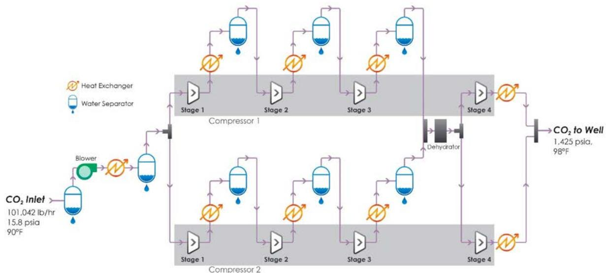
Figure 3-7: CO<sub>2</sub> Compression Train Process Simulation Flow Sheet for the Illinois Basin – Decatur Project
