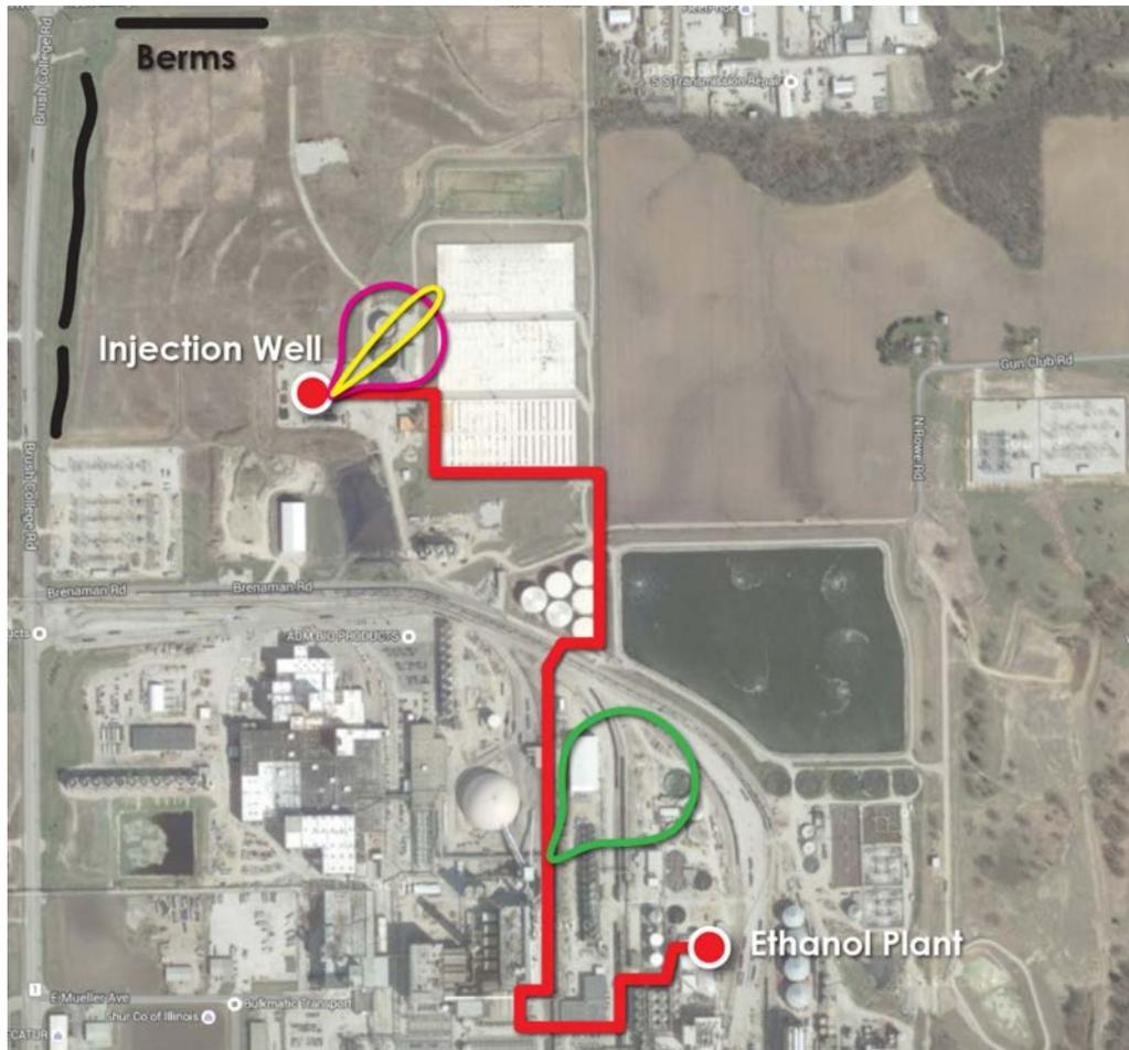
Figure 3-8: Plan view of the Decatur site showing release contours from the wellhead end of the pipeline and from the middle of the pipeline. The Yellow (1.22 m elevation – downwards impinging), pink (1.22 m – vertically downwards) releases are at the wellhead end of the pipeline. The green (4.82 m) release is in the middle of the pipeline. The contours are measured to a concentration of 40,000 ppm and the wind direction is from the south west.
