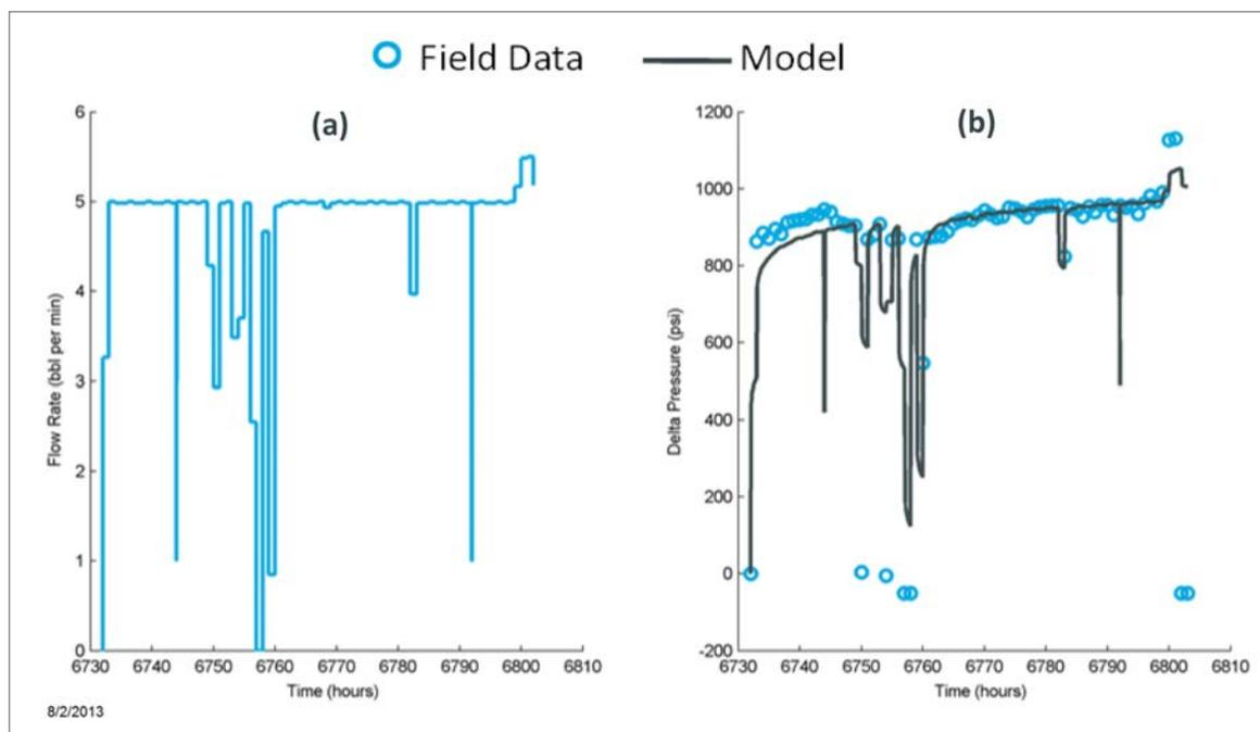
Figure 3-2: Segment analysis of a brine disposal well with an average injection rate of 4.72 bb/min depicting (a) average hourly injection rate calculated from field data and (b) field data delta pressure response and model pressure response match at transmissivity,  $T=11,000$  mD-ft/cP
