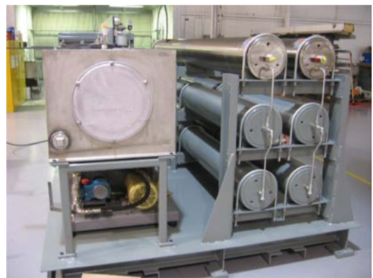
125-gal annular fluid tank (top left) and annular fluid pumps (bottom left)
