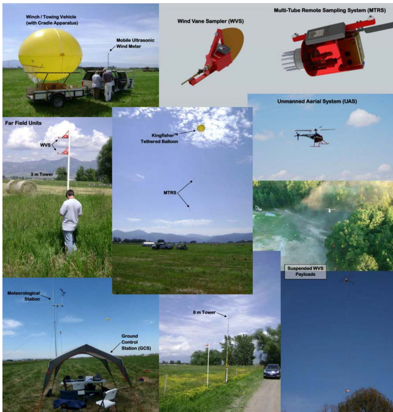
Figure 8: MTRS and WVS Systems for Atmospheric PFT Tracer Monitoring
