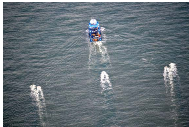
FIGURE 12. AERIAL PHOT OF THE R/V BROOKS MCCALL DURING ACTIVE HR3D (P-CABLE) SEISMIC ACQUISITION IN OCTOBER 2013, OFFSHORE SAN LUIS PASS, TEXAS.
