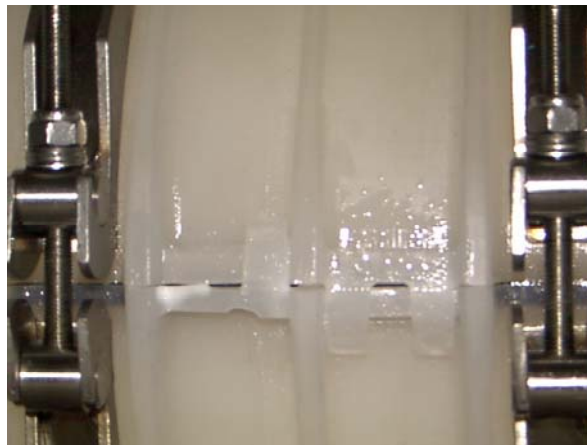
Figure 10. Sustained pressure testing to verify leak tightness of proposed seal design at 60 psig internal pressure
