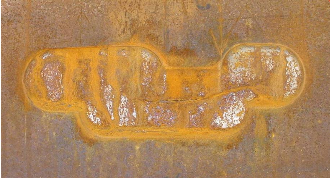
Figure 167 - Test 09 Damage after Burst Test
