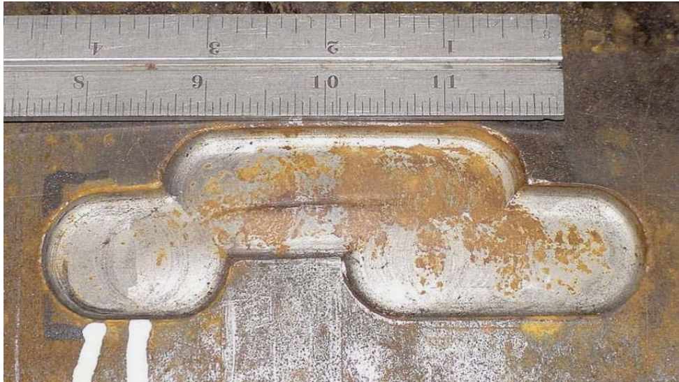
Figure 168 - Test 10 Damage after Burst Test
