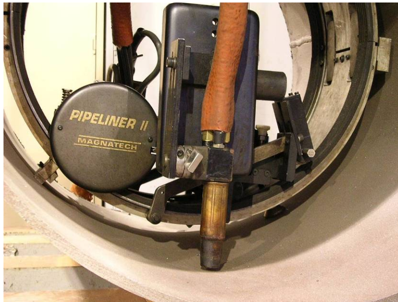
Figure 27 - Magnatech Pipeliner II Welding Tractor
