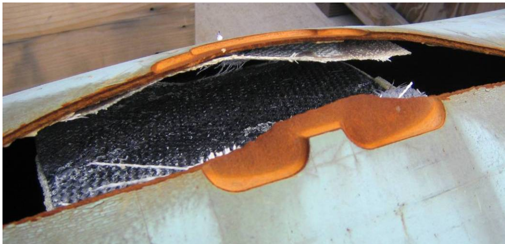
Figure 153 - Test 04 Failure Initiation Site
