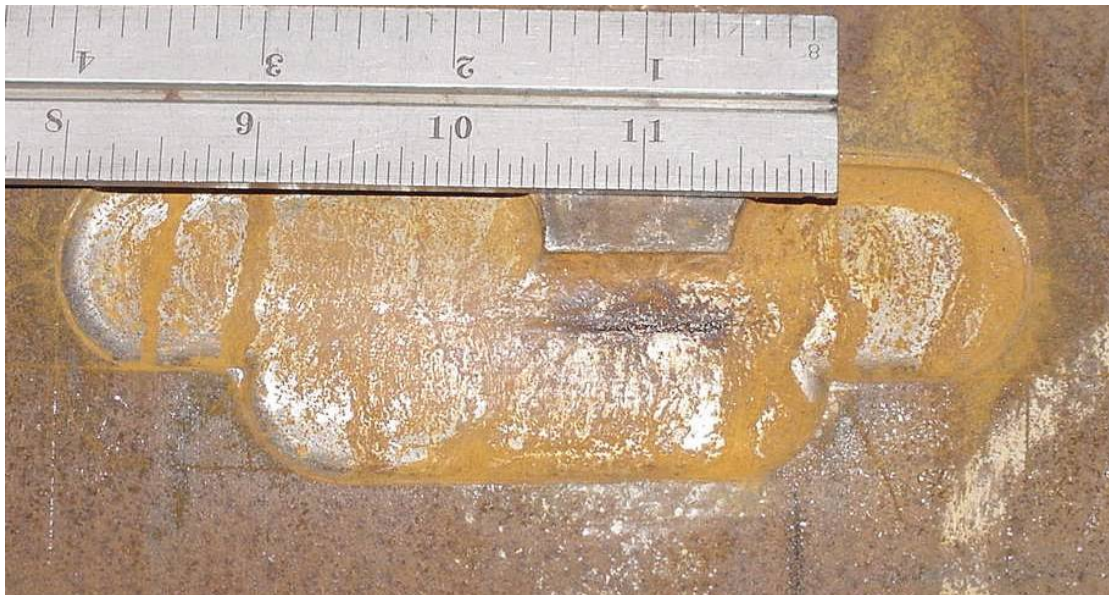
Figure 170 - Test 11 Damage after Burst Test
