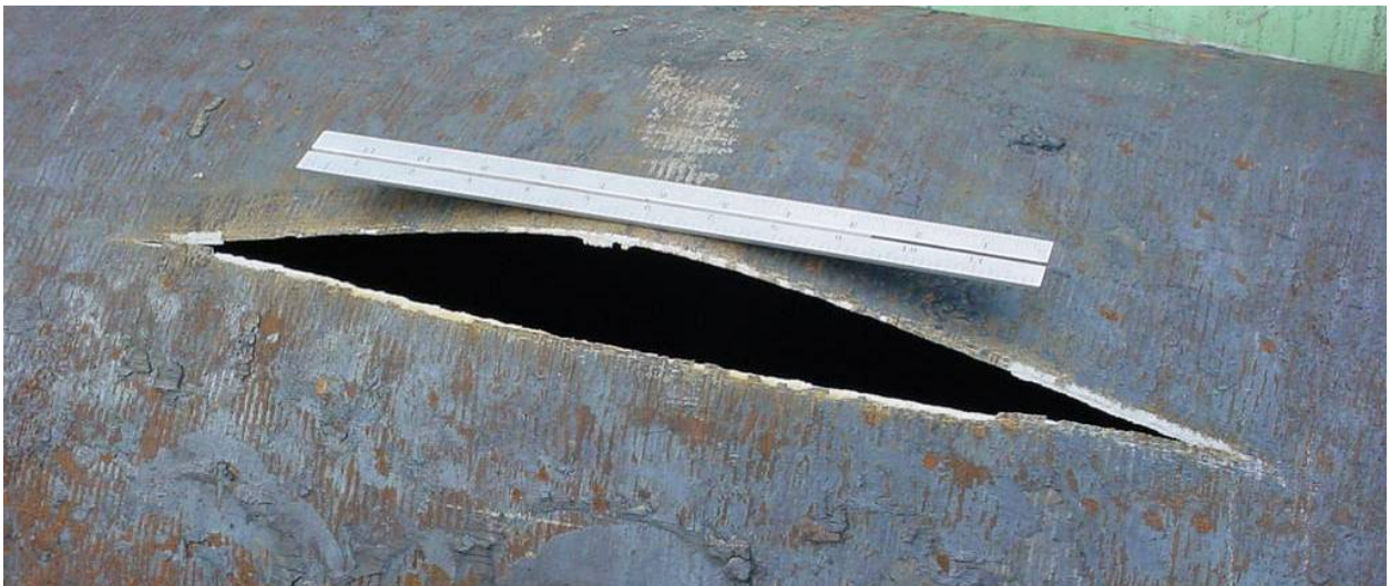
Figure 96 - 558.8 mm (22 in.) Virgin Pipe After Burst Testing
