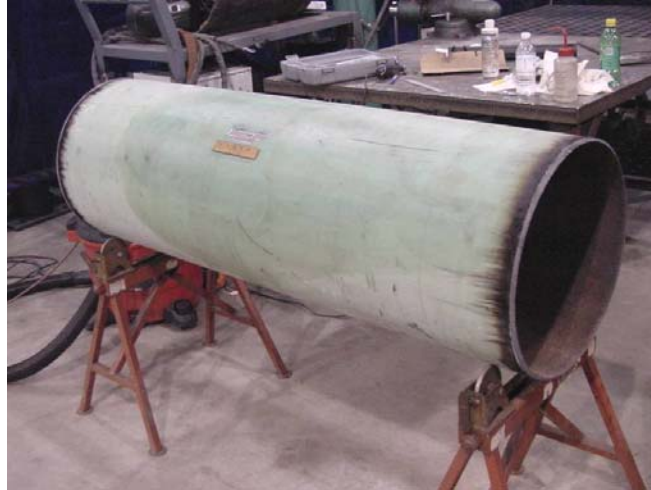
Figure 35 - Pipe Section Used for Carbon Fiber Patch Test 04
