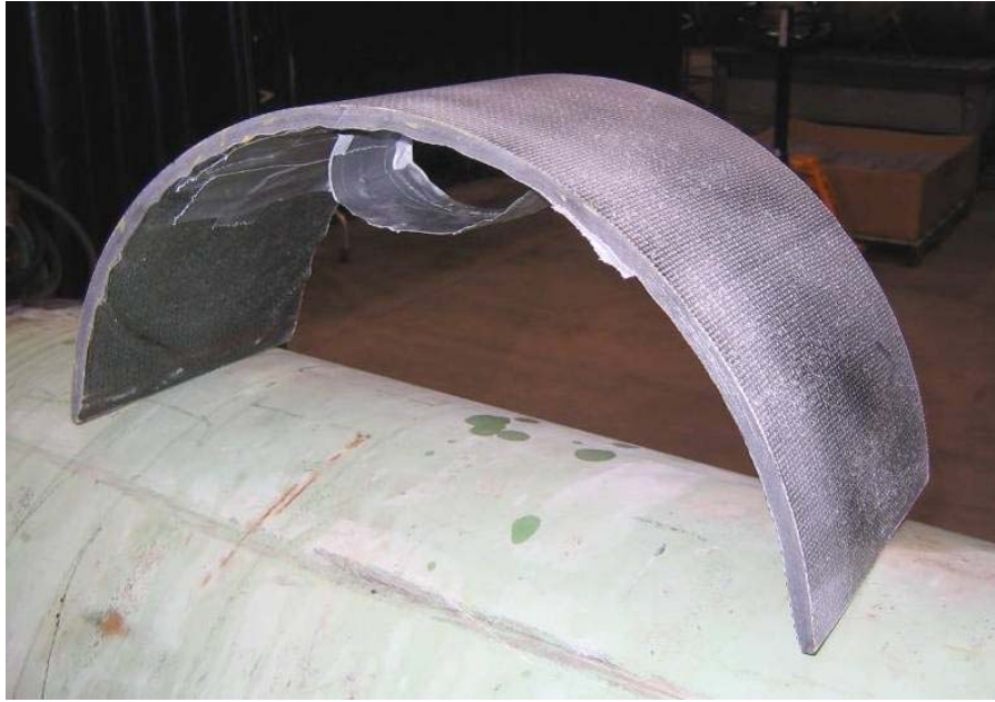
Figure 41 - Completed Test 04 CF Patch with Grit-Blasted OD
