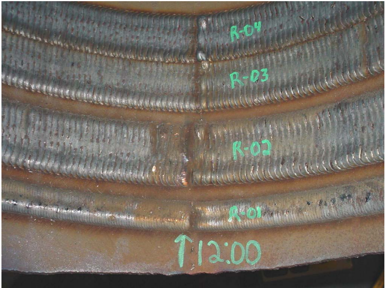
Figure 110 - Tests R-01 - R-04 at 12:00 (Note the Poor Tie-Ins for R-01 through R-03)
