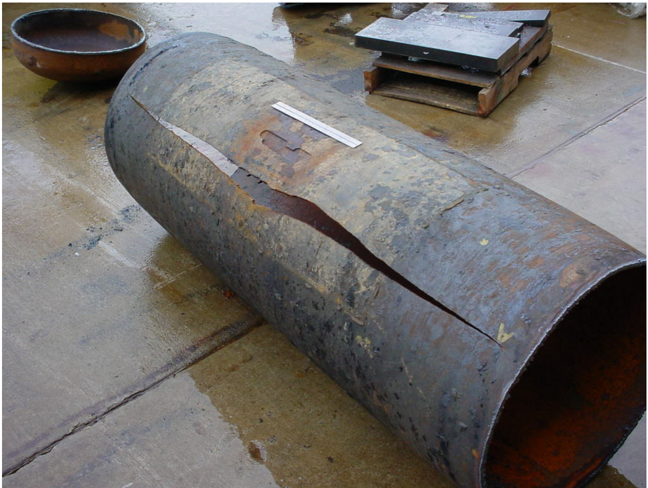
Figure 130 - Test 01 Pipe Section After Hydrostatic Burst Test
