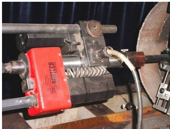
Figure 23 - Bortech Motion Mechanism for Continuous Spiral Deposition
