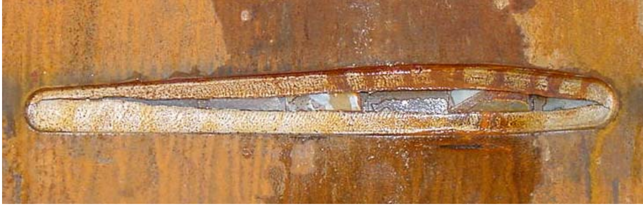
Figure 176 - Test 14 Damage after Burst Test
