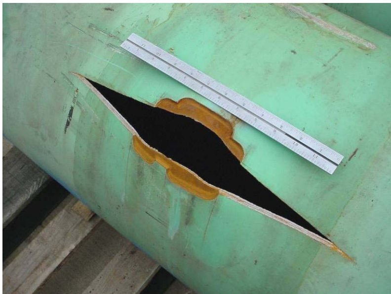
Figure 95 - 508.0 mm (20 in.) Pipe with Un-Repaired Damage After Burst Testing
