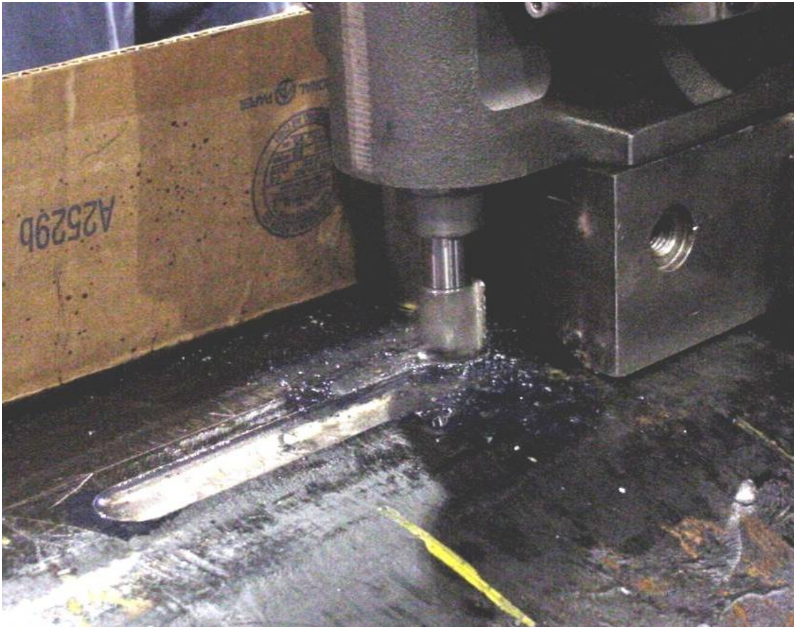
Figure 11 - Milling Machine Set-Up Used to Simulate Corrosion Damage on Pipe Sections
