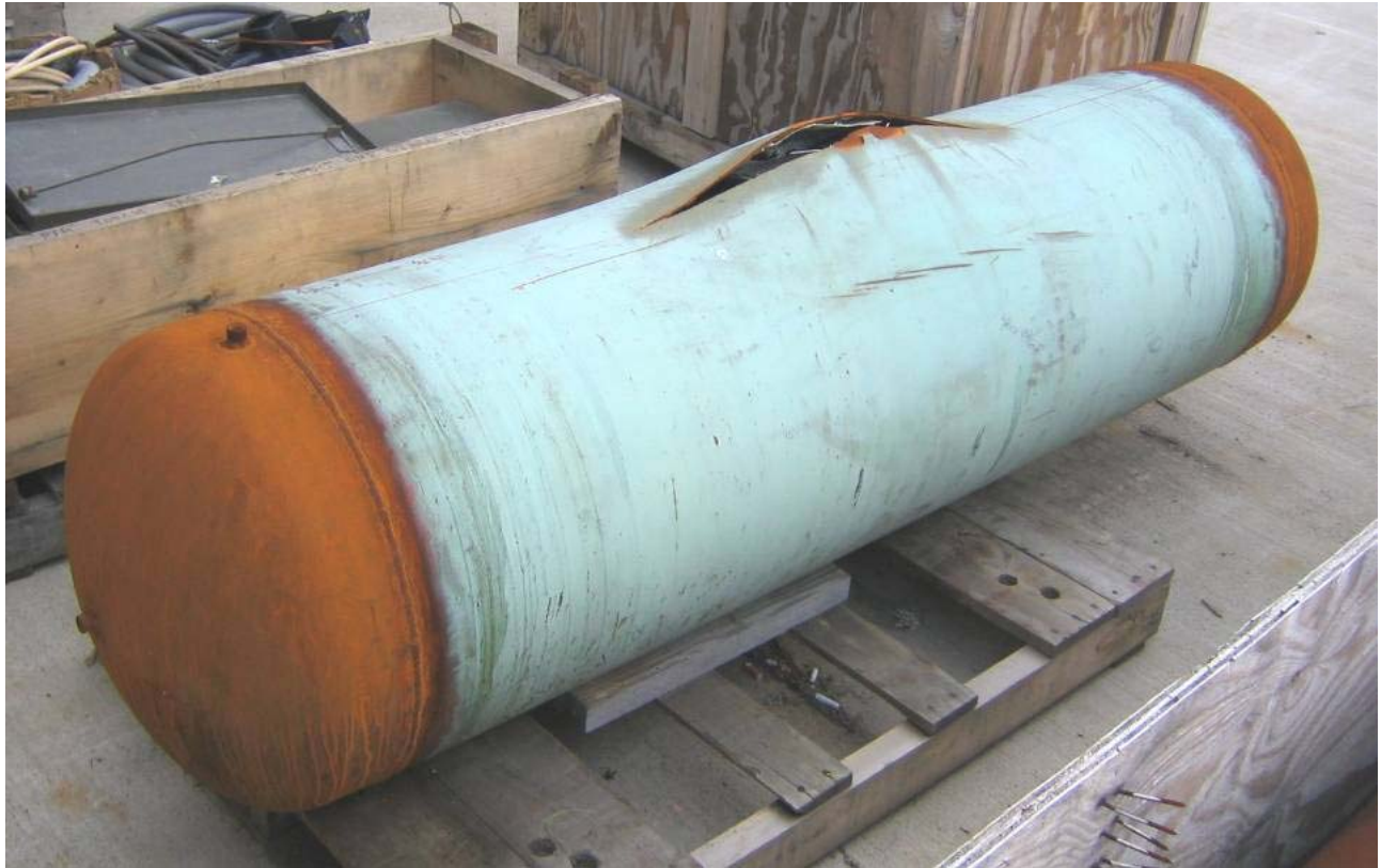
Figure 152 - Test 04 Pipe With CF Patch Repair After Burst Test
