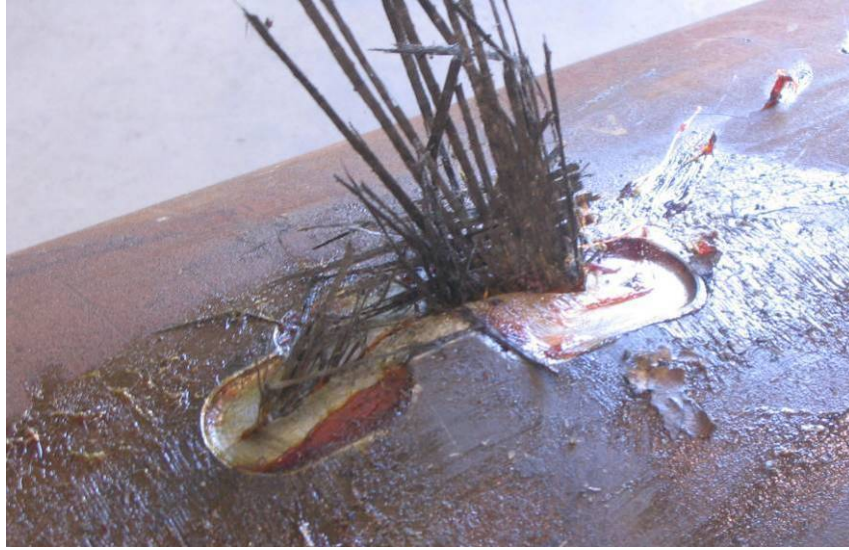
Figure 158 - Test 06 Damage after Burst Testing
