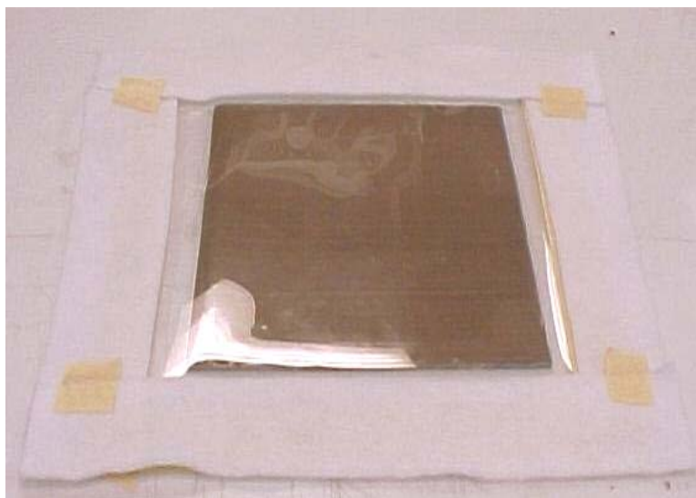
Figure 51 - Rim of Breather Added \cong 76.2 mm (3 in.) Wide
