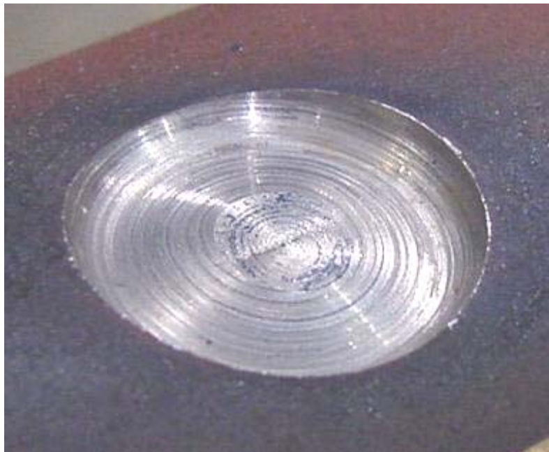
Figure 149 - Test 03 Pipe with GF Liner Repair of Short/Deep Damage after Burst Test
