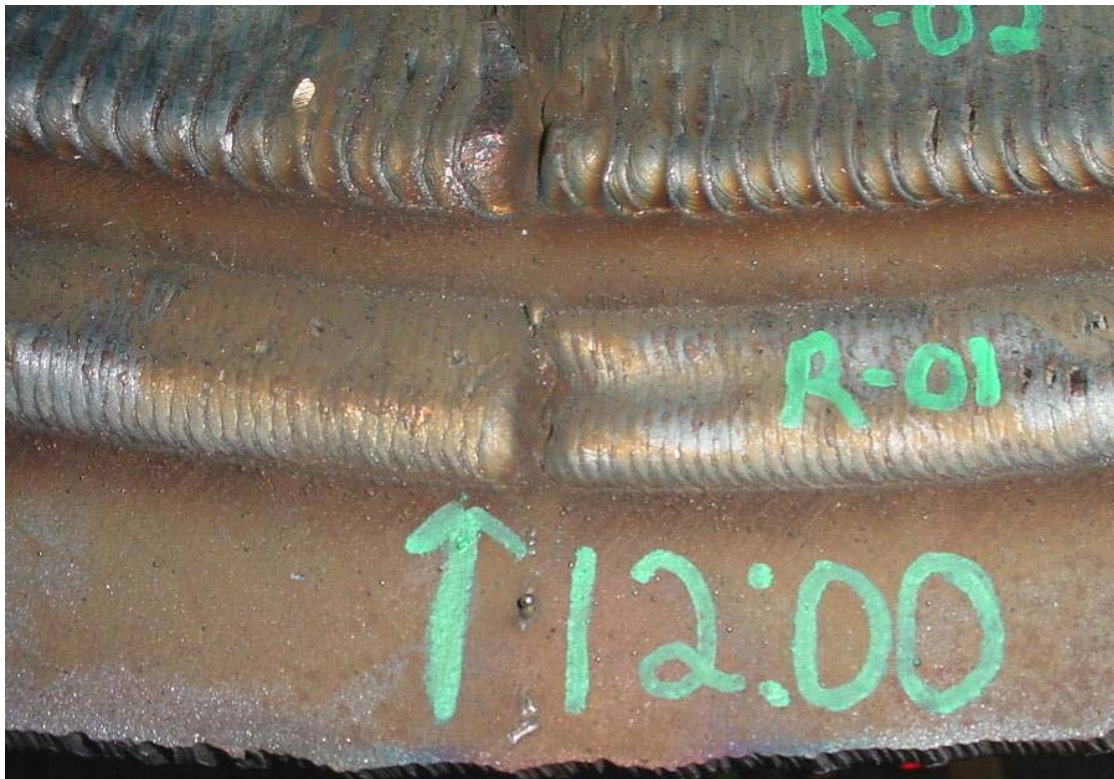
Figure 111 - Test R-01 at 12:00 Show Poor Stop-Start Tie-In
