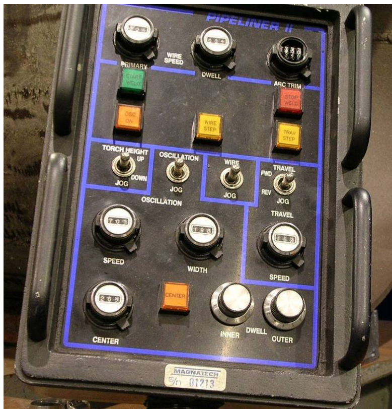
Figure 28 - Magnatech Control Pendant
