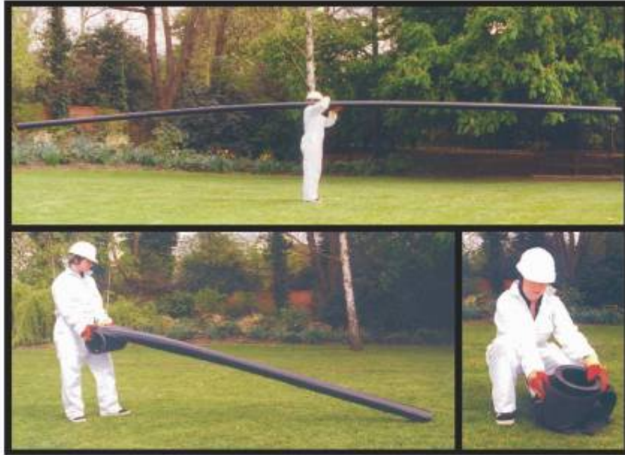
Figure 145 - RolaTube Bi-Stable Reeled Composite Material
