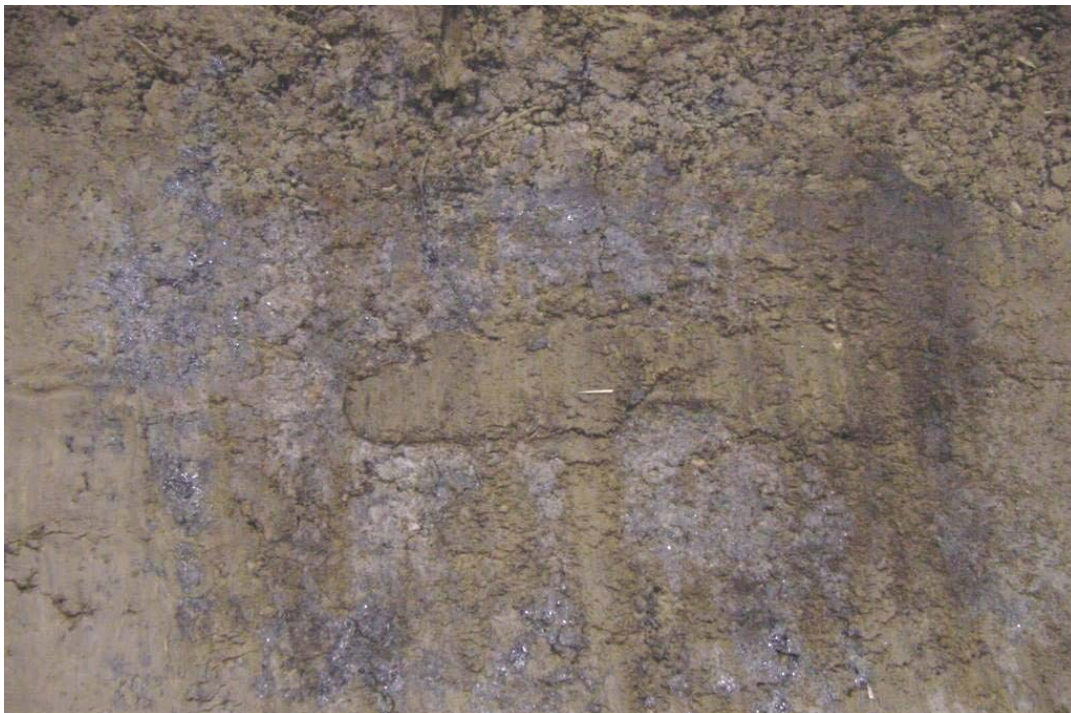
Figure 127 - Soil in Contact With Pipe During Weld Repair Test 01
