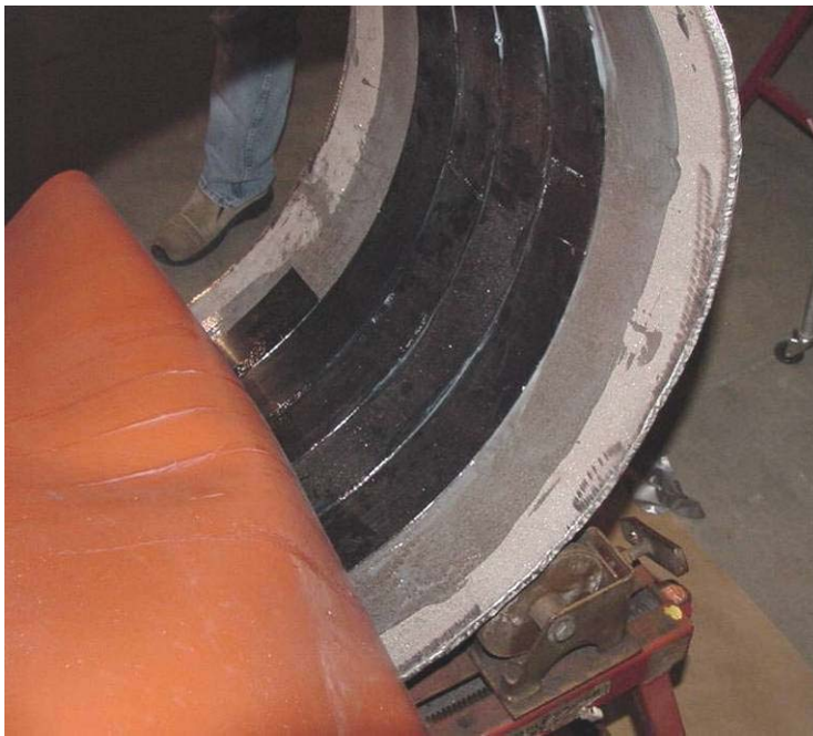
Figure 67 - Helically Wound Steel Strip Expanded to Fit Pipe ID (similar to Test 09)
