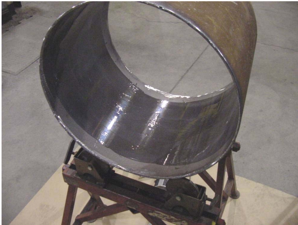
Figure 65. ID of Demonstration Pipe (similar to Test 09) with 3M DP460 Epoxy Applied
