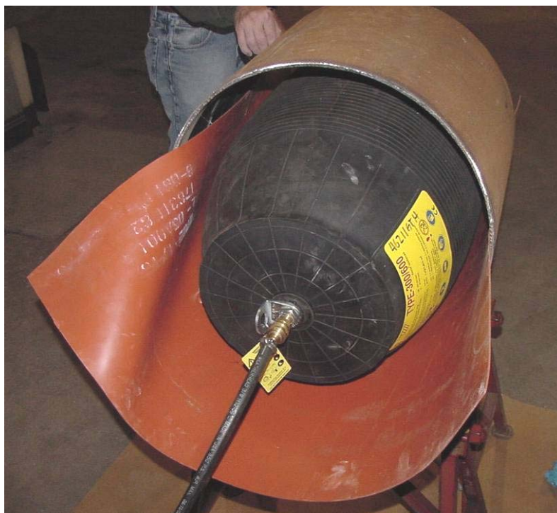
Figure 68 - Inflatable Bladder Inserted in Pipe (similar to Test 09)
