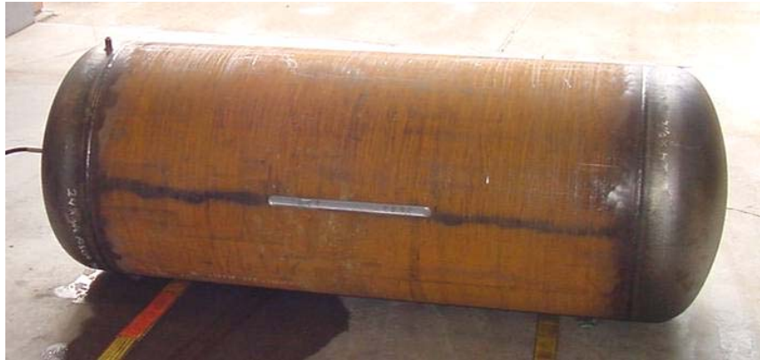
Figure 12 - End Caps Welded on Pipe Section in Preparation for Hydrostatic Testing
