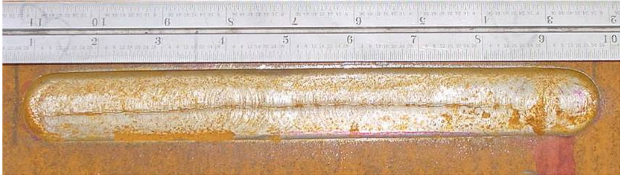
Figure 171 - Test 12 Damage after Burst Test
