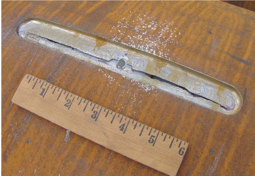
Figure 173 - Test 13 Damage after Burst Test
