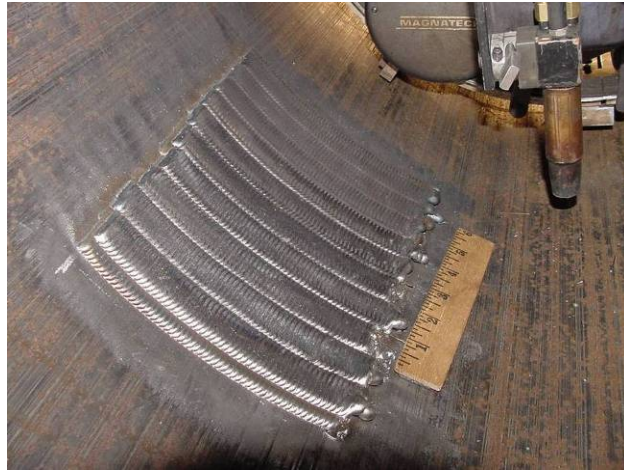
Figure 124 - Finished Weld Layer 2 of Test 01
