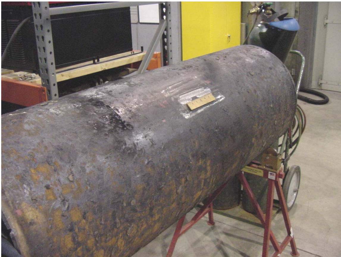
Figure 115 - Short/Deep Simulated Corrosion on 558.80 mm (22 in.) Pipe for Test 01
