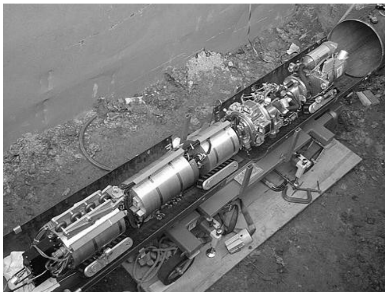
Figure 4 - Internal Pipeline NDE System (IPNS)
