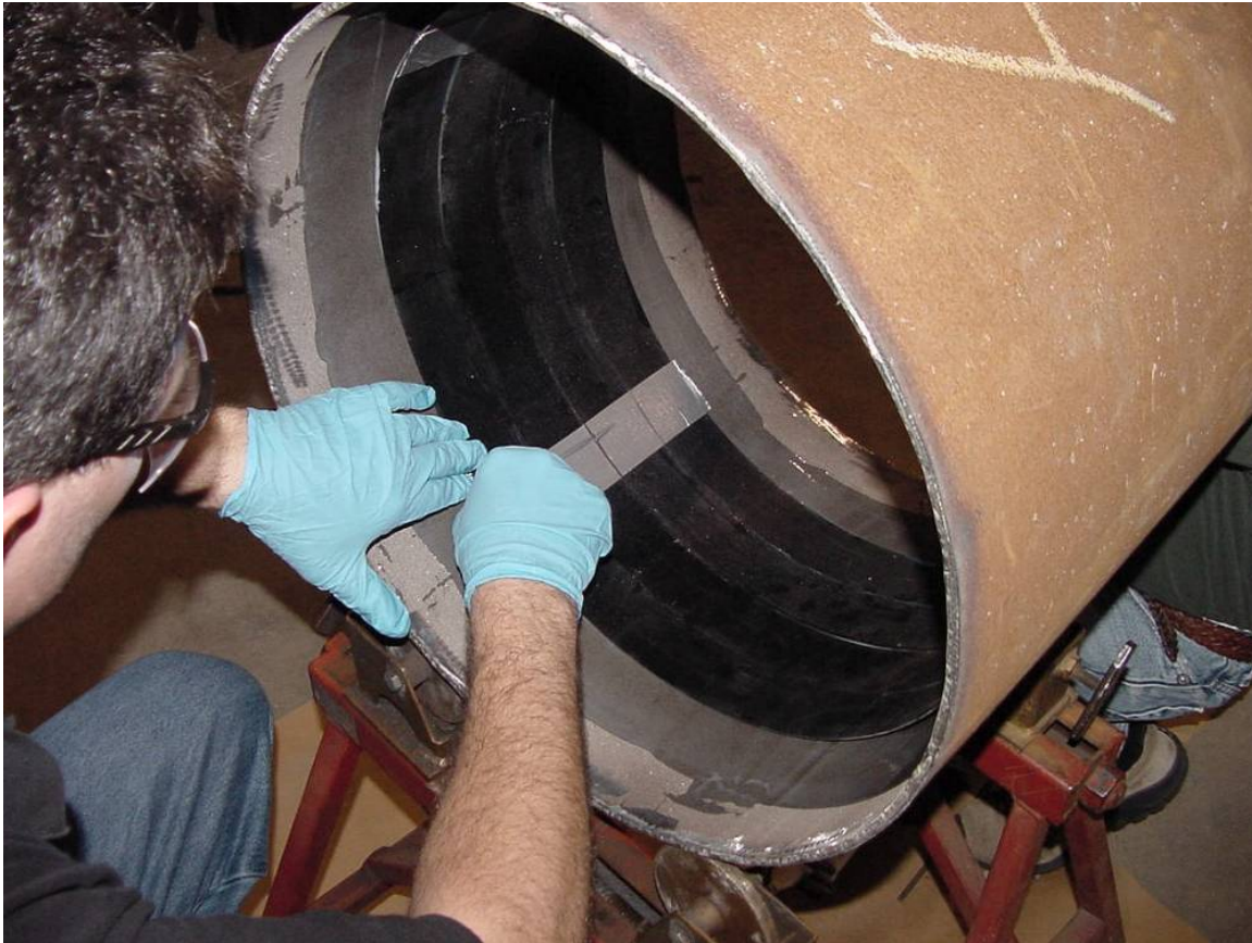
Figure 66 - Helically Wound Steel Strip Inserted into Pipe (similar to Test 09)
