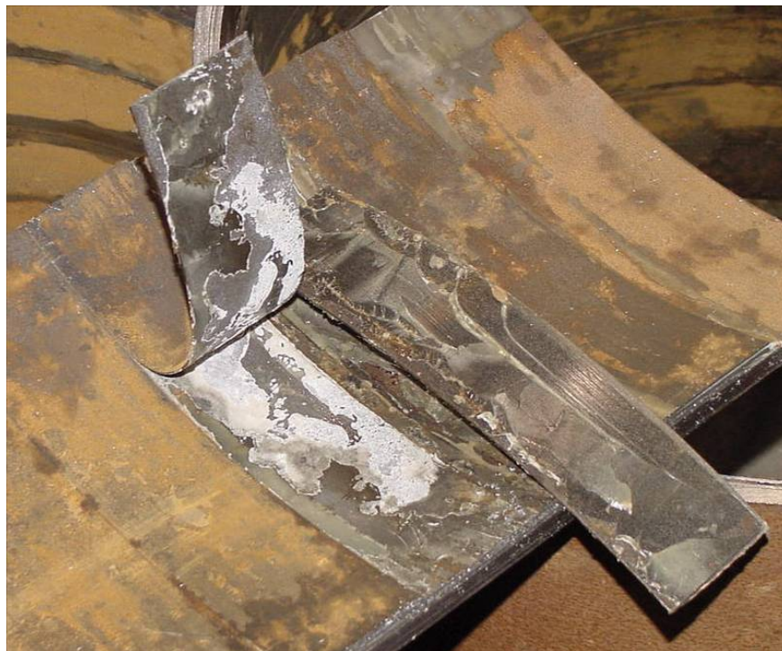
Figure 169 - Large Number of Voids in Urethane Adhesive from Test 10
