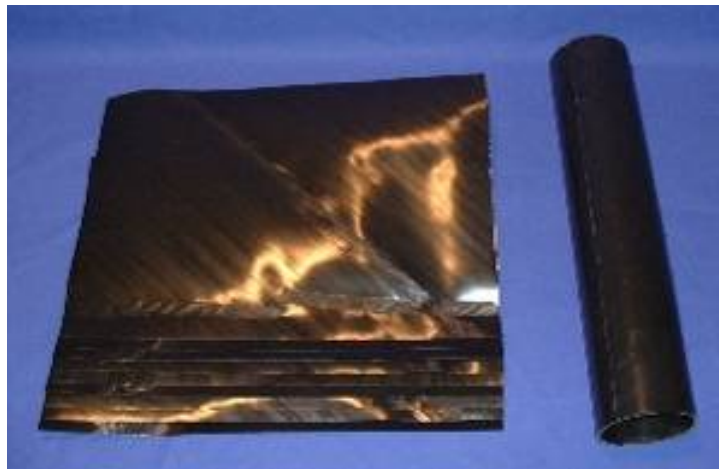
Figure 30 - Lay-Up and Forming of GF-Reinforced Composite Liner
