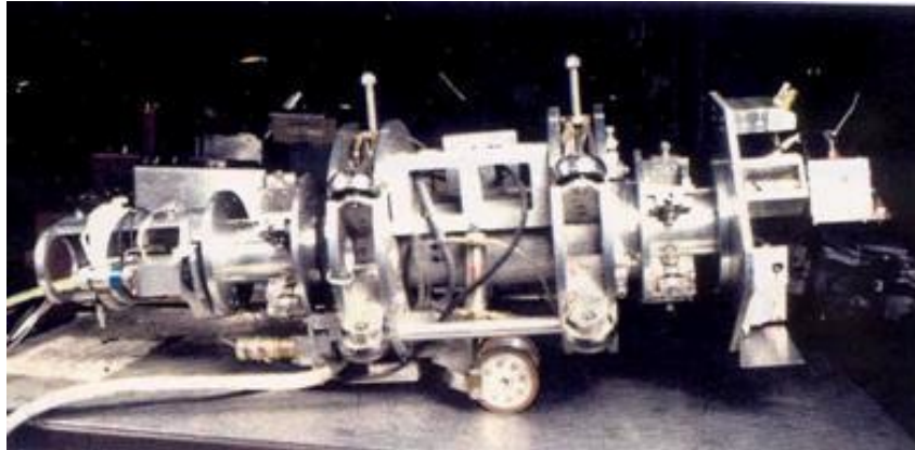
Figure 3 - Osaka Gas System Robotic Welding System
