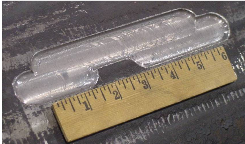
Figure 18 - Short/Deep Simulated Corrosion Damage for 558.8 mm (22 in.) Pipe
