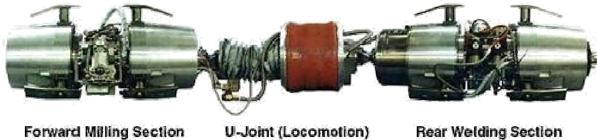
Figure 5 - Welding and Inspection Steam Operations Robot (WISOR)
