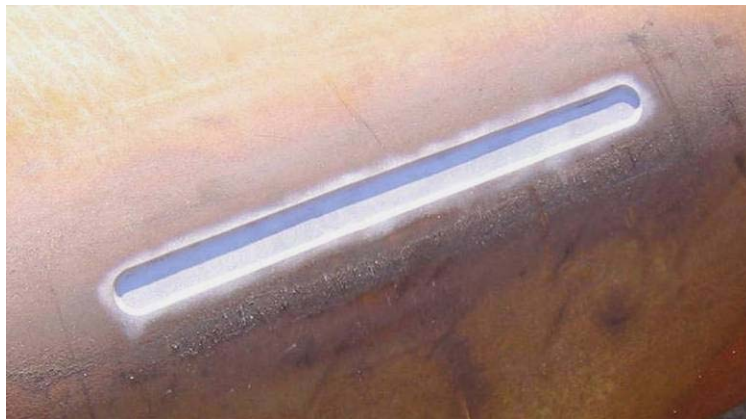
Figure 17 - Long/Shallow Simulated Corrosion Damage for 508 mm (20 in.) Pipe
