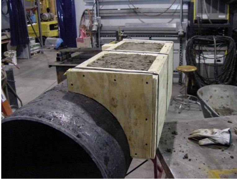
Figure 116 - Soil Box for Weld Deposition Repair Test 01
