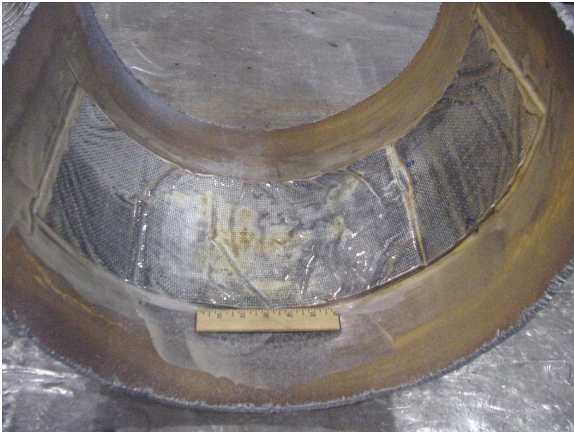
Figure 47 - Test 05 "Pressure Bandage" CF Patch
