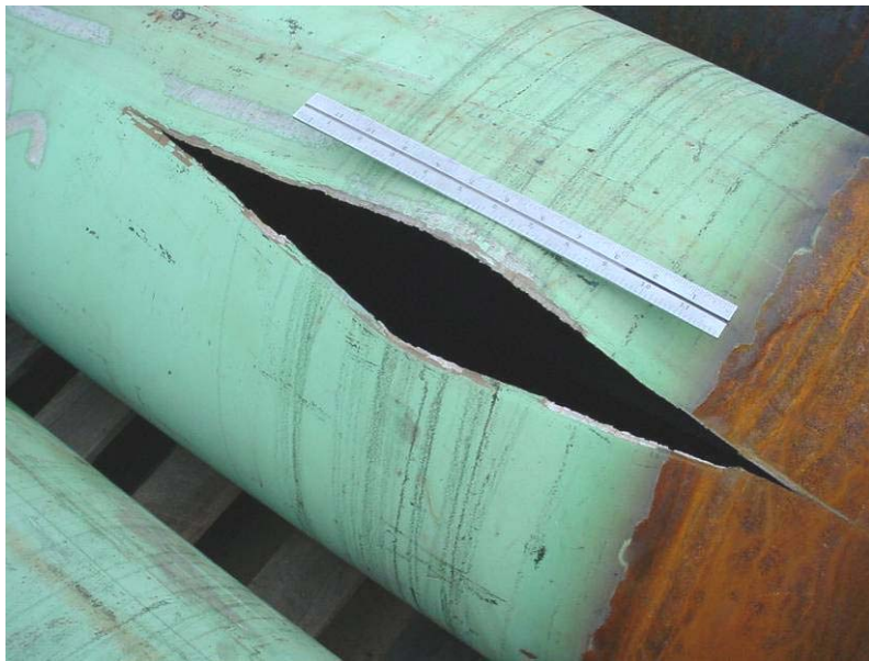
Figure 94 - 508.0 mm (20 in.) Virgin Pipe After Burst Testing
