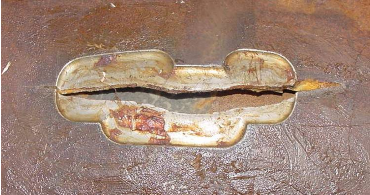
Figure 163 - Test 08 Damage after Burst Test
