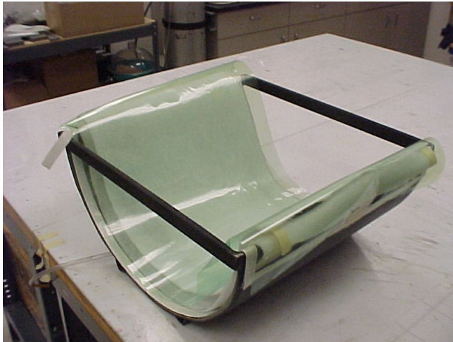
Figure 40 - Vacuum Bag Film Draped Over Entire Pack
