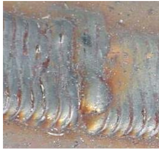
7:00 – Bad Appearance Due Robot Program Error
