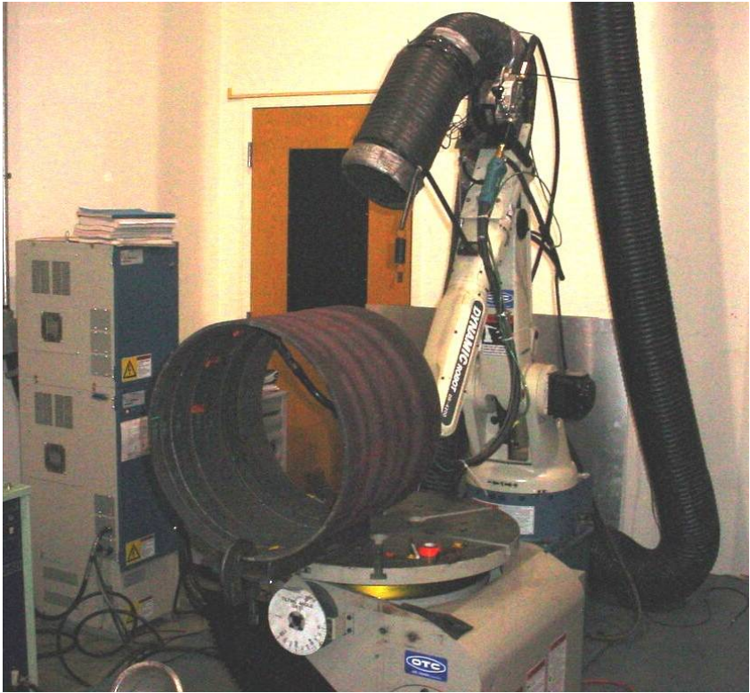
Figure 25 - OTC Robot Set-Up for Internal Welding
