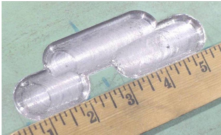
Figure 16 - Short/Deep Simulated Corrosion Damage for 508 mm (20 in.) Pipe
