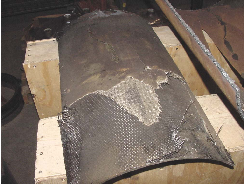
Figure 161 - Test 07 Patch after Burst Testing
