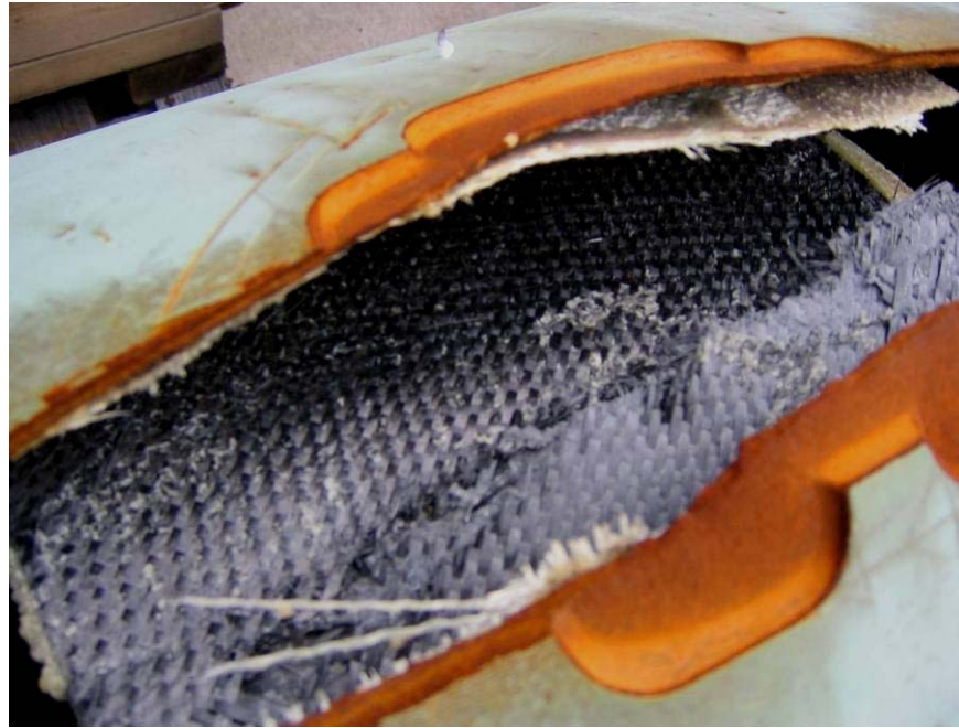
Figure 154 - Magnified Test 04 Failure Initiation Site
