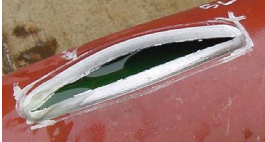
Figure 92 - 114.3 mm (4.5 in.) Pipe with Un-Repaired Long/Shallow Damage after Burst Test
