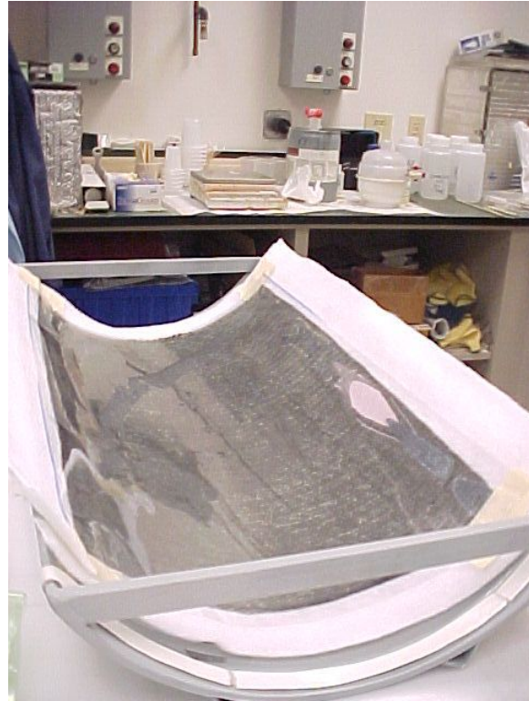
Figure 49 - Test 07 CF Patch for Long/Shallow Defect Evaluation
