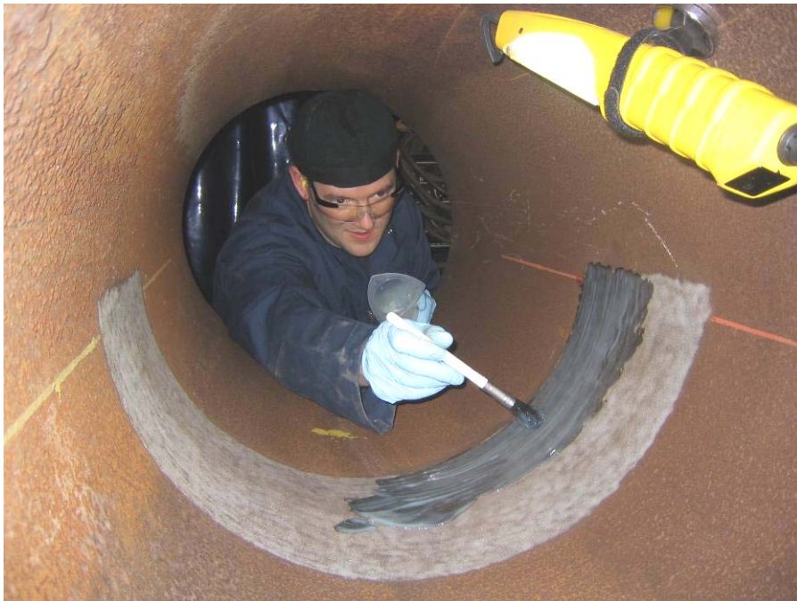
Figure 42 - Application of 3M DP460 Adhesive to Grit-Blasted ID of Test 04 Pipe
