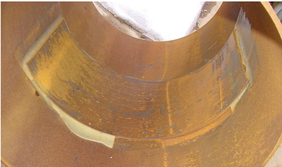
Figure 164 - Inside of Test 08 Pipe Section After Burst Test
