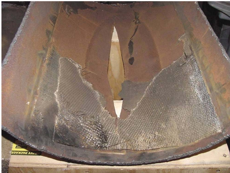
Figure 160 - Inside Surface of Test 07 Pipe Section After Burst Test
