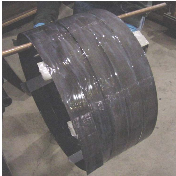
Figure 64 - Test 09 Helically Wound Steel Strip with 3M DP460 Epoxy Applied
