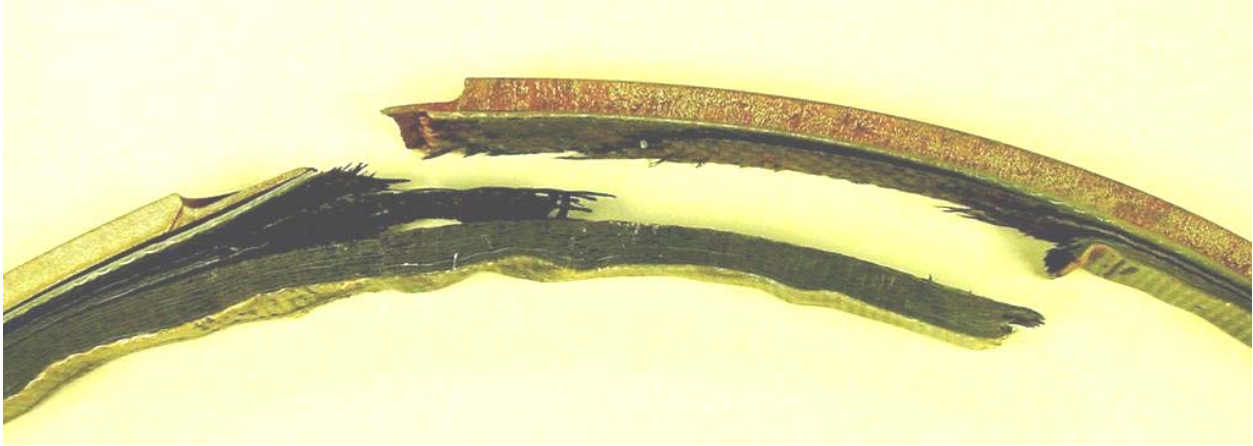
Figure 156 - Failure of Test 05 Pipe and Composite Repair
