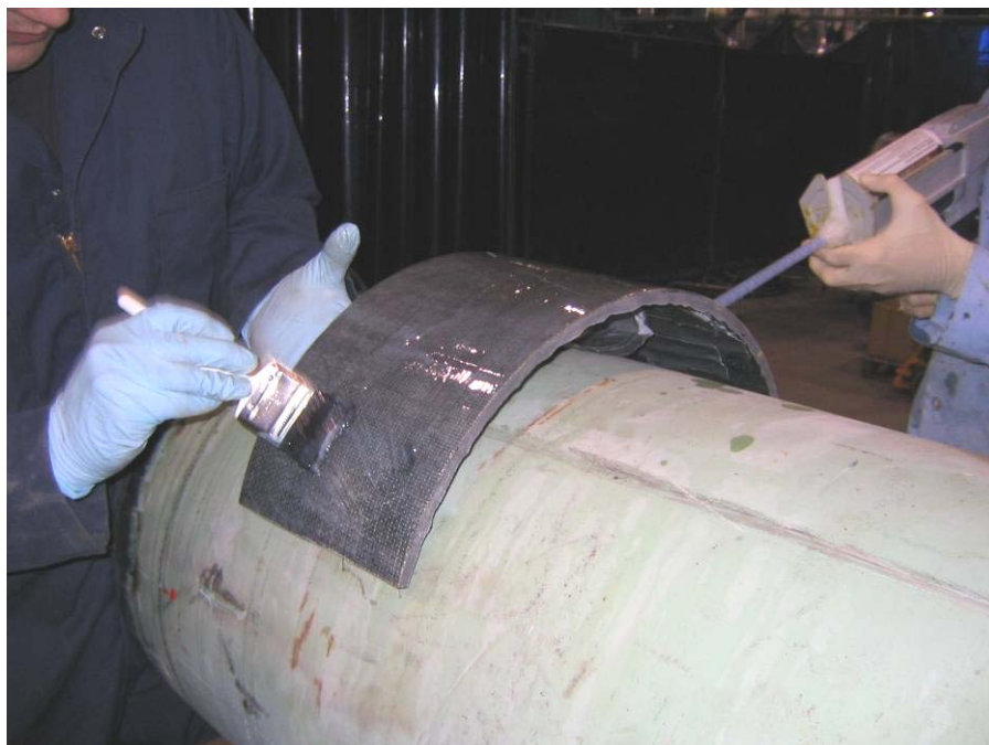
Figure 43 - Application of Adhesive to Test 04 CF Patch
