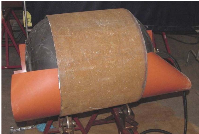
Figure 69 - Bladder Pressurized to 206 kPa (30 psi) (similar to Test 09)
