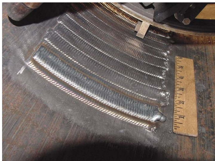
Figure 123 - First Pass of Weld Layer 2 for Test 01
