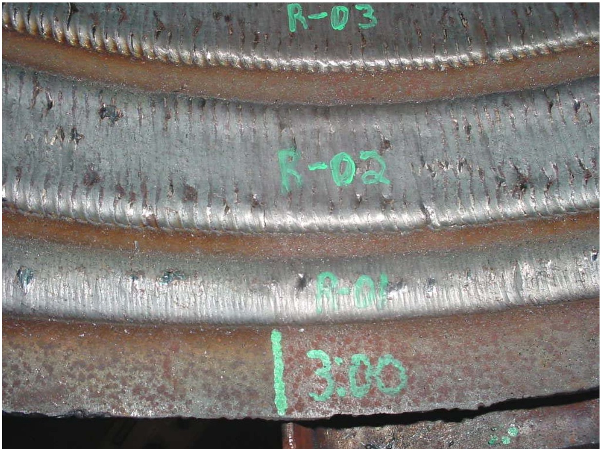
Figure 113 - Tests R-01 and R-02 at 3:00 Showing Steady-State Bead Shape
