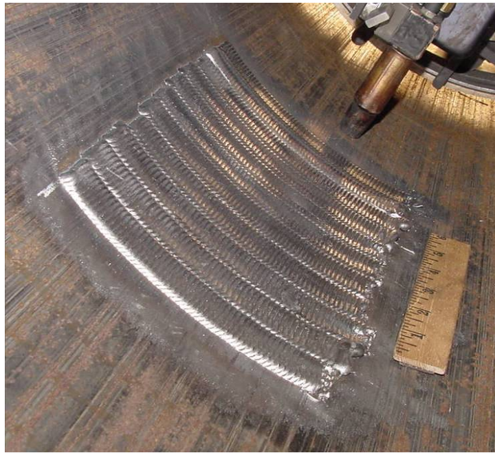
Figure 122 - Completed Weld Layer 1 for Test 01
