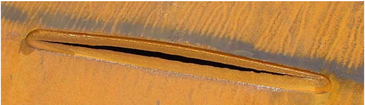
Figure 98 - 609.6 mm (24 in.) Pipe with Un-Repaired Extra Long/Shallow Damage After Burst Testing
