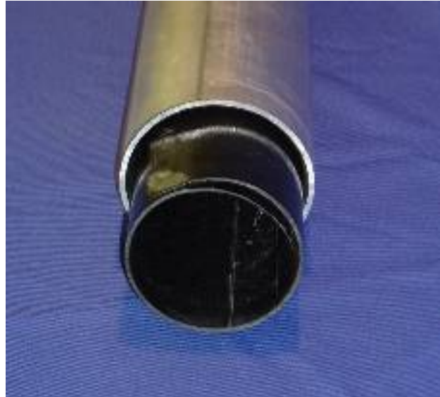
Figure 31 - Insertion of GF Liner into 114.3 mm (4.5 in.) Diameter Pipe
