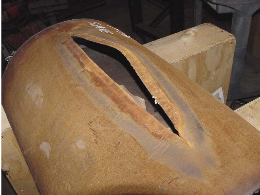
Figure 159 - Test 07 Damage After Burst Test
