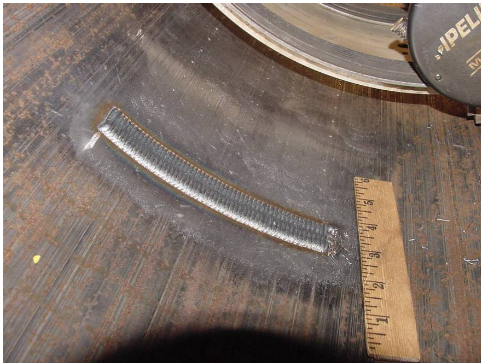
Figure 119 - First Pass of Weld Layer 1 for Test 01
