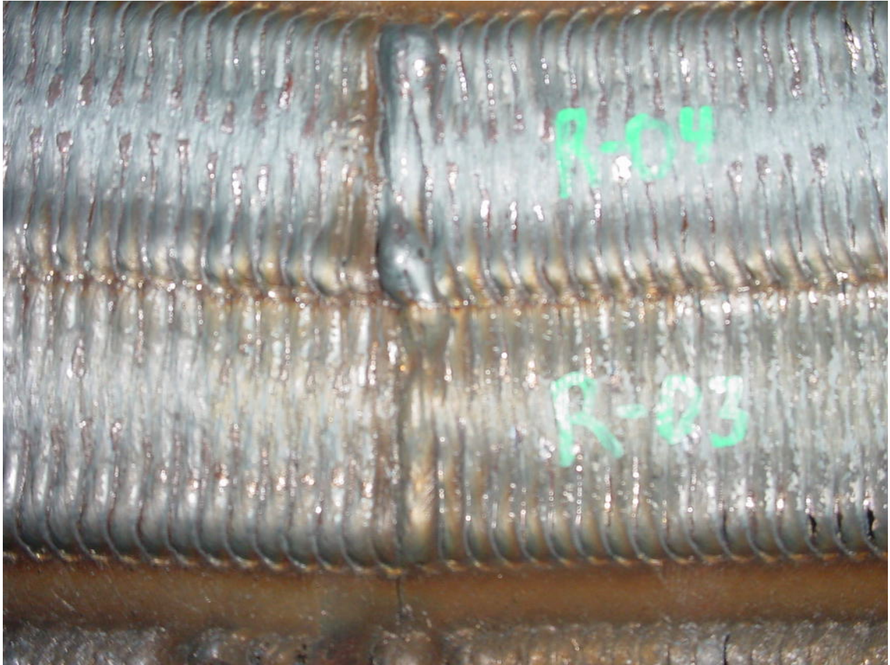
Figure 112 - Tests R-03 and R-04 at 12:00 Show Better Stop-Start Overlap
