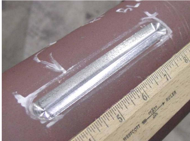
Figure 14 - Long/Shallow Simulated Corrosion Damage for 114.3 mm (4.5 in.) Pipe
