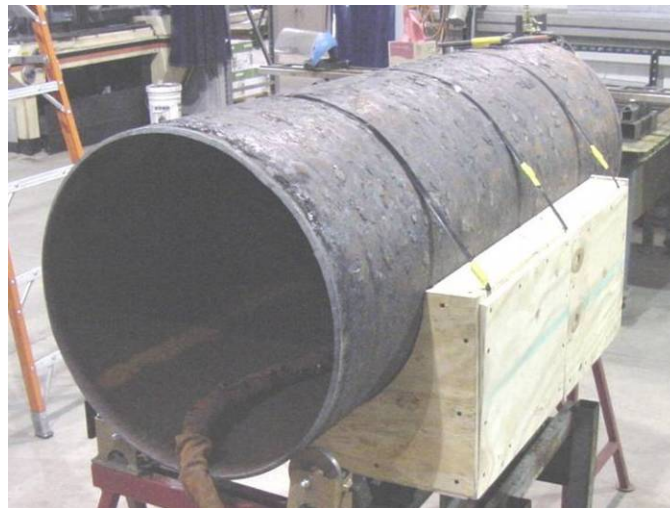
Figure 117 - Orientation of Pipe Section with Dirt Box for Weld Deposition Repair Test 01
