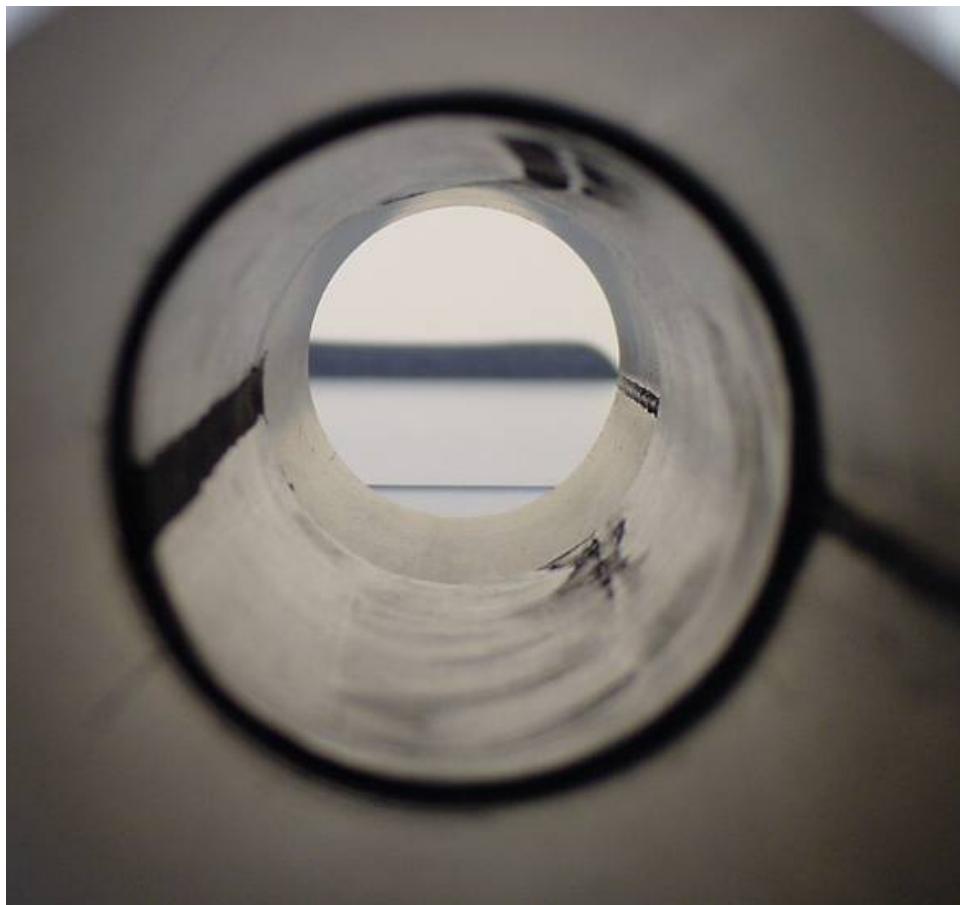
Figure 34 - GF Liner Installed in 114.3 mm (4.5 in.) Diameter Pipe
