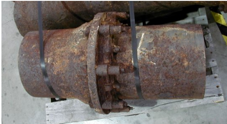
Figure 21. Sample Cast-Iron Joint for Full-Function Tests of Patching Module
