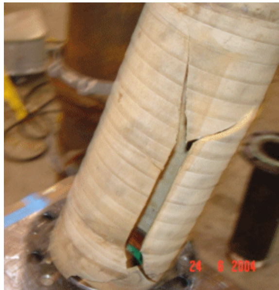
Figure 16. Ruptured Inflation Bladder
