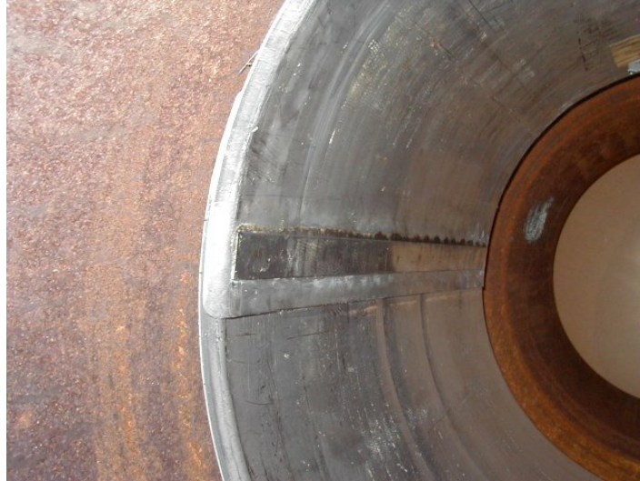
Figure 22. Final Patch Design Set in Test Joint
