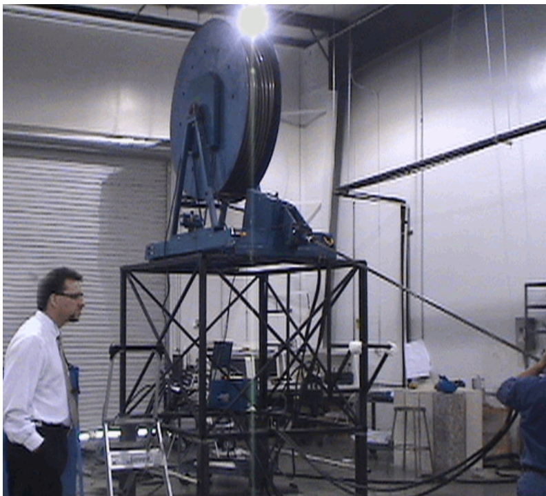
Figure 4. Coiled-Tubing Locomotion Unit
