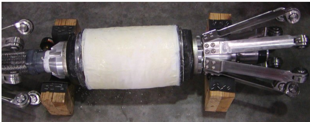
Figure 12. Prepared Patch on Bladder
