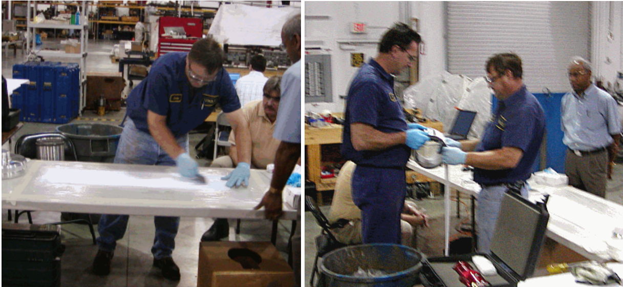
Figure 54. Preparing Patch for Setting in Pipe
