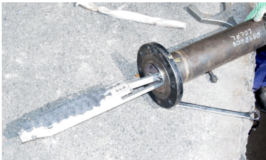
Figure 60. Magnet Assembly for Removing Filings
