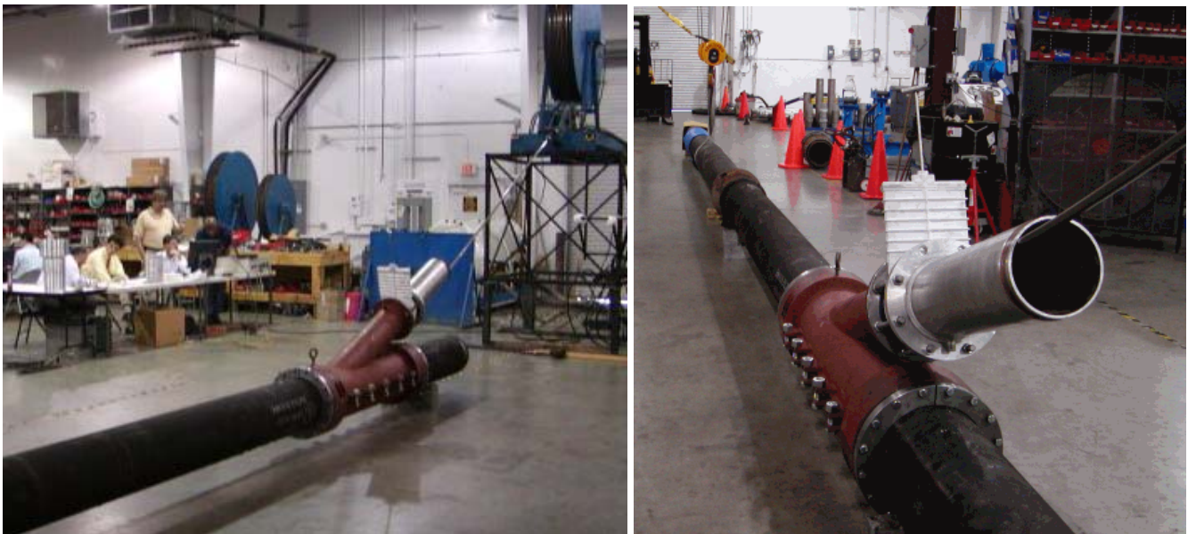
Figure 50. Shop Tests – Entry Fitting, CT Unit and Pipeline
