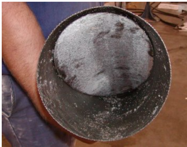
Figure 47. Hole Saw with Captured Coupon
