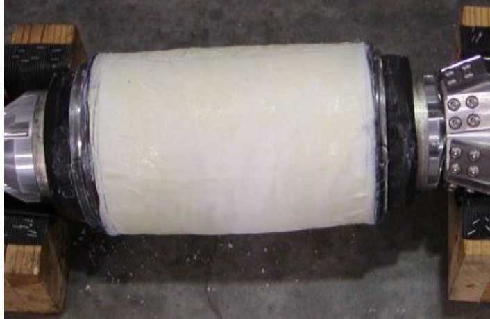
Figure 7. Complete Repair Sleeve with Epoxy Applied
