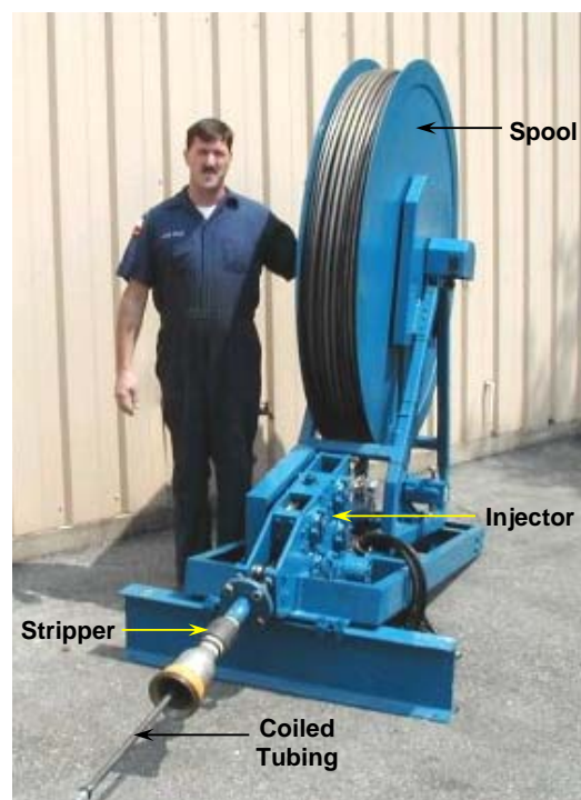
Figure B-1. CT Delivery System
