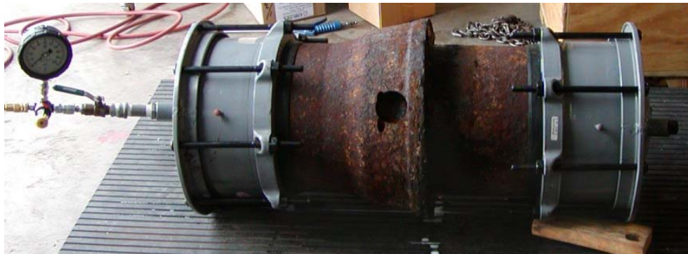
Figure 18. Cast-Iron Joint Tested for Leaks
