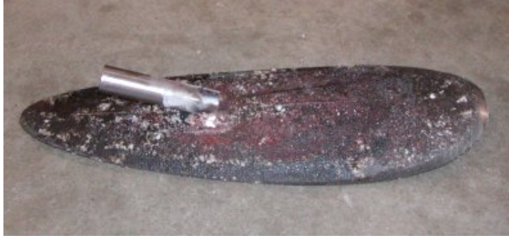
Figure 48. Pipe Coupon after Retrieval
