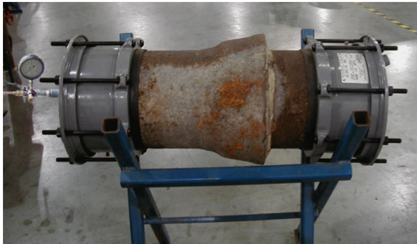
Figure 57. Patched CI Joint Tested for Leaks
