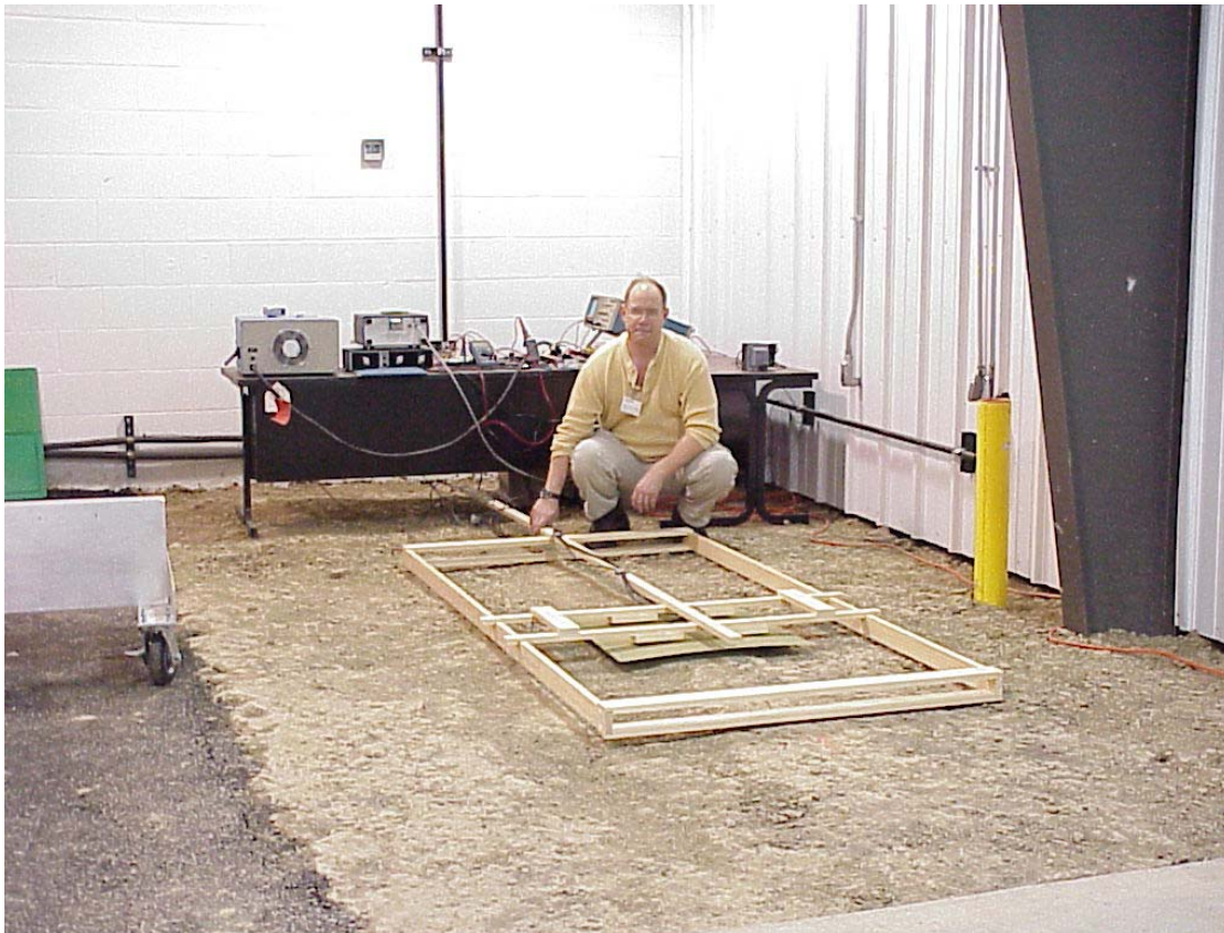
Figure 4. 4-Element CT Array in GTI Soil Lab
