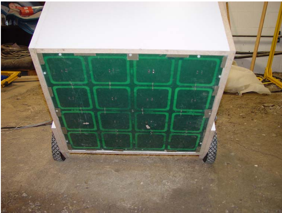
Fig. 29. Bottom side of CT sensor array mounted to cart.
