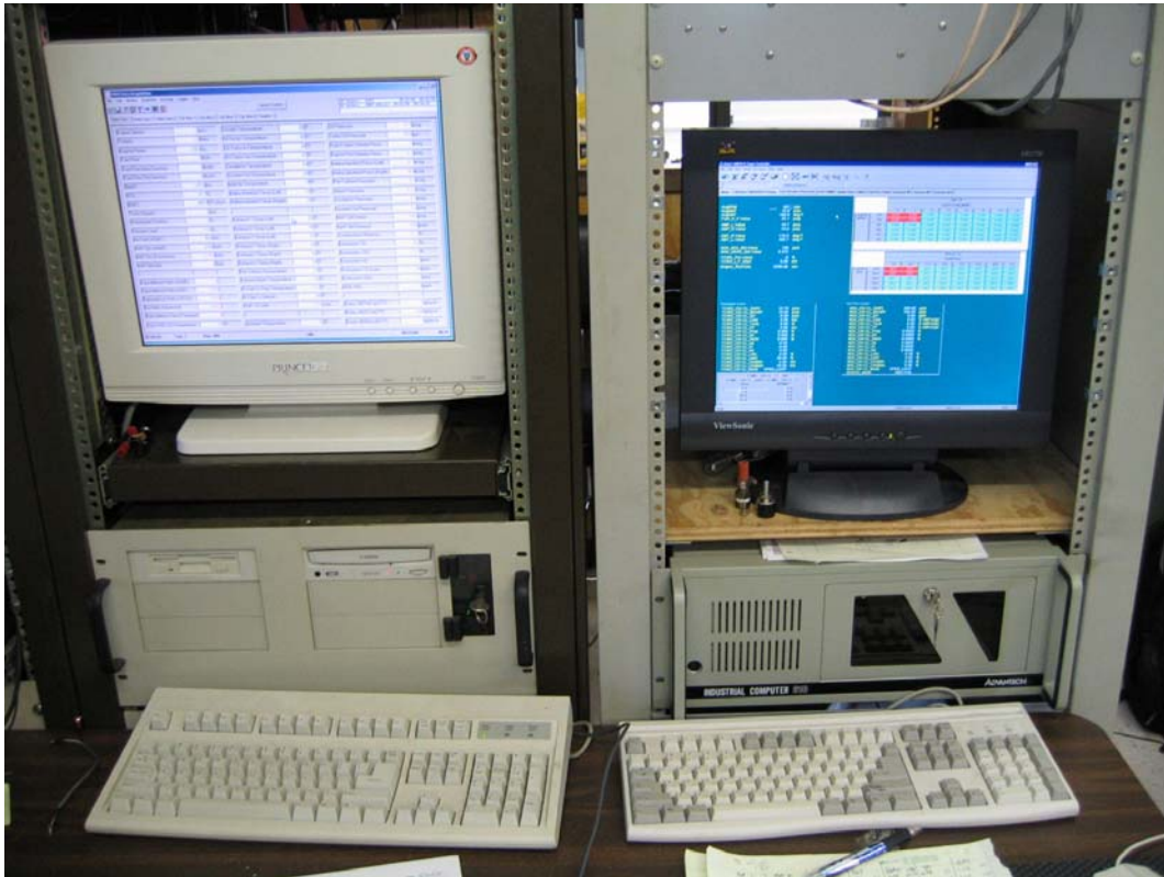
Figure 6.2. Photograph of RPECS and Data Acquisition System
