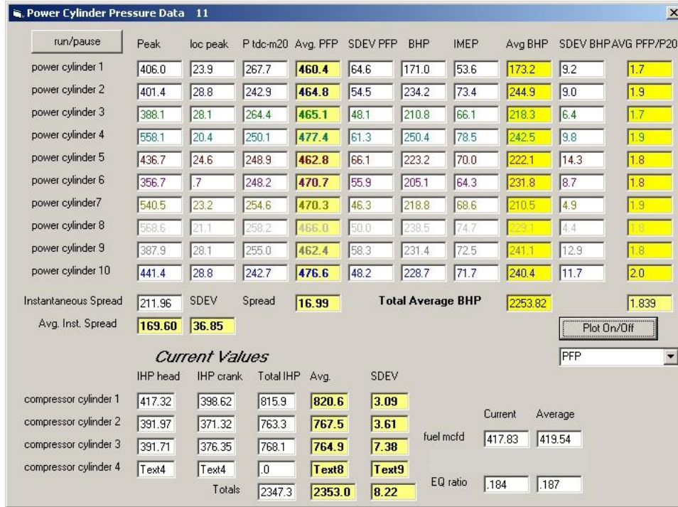
Figure 5-3. Snapshot of On-Site Real-Time Calculations; (Williams Station 40 (Sour Lake); August 2004)
