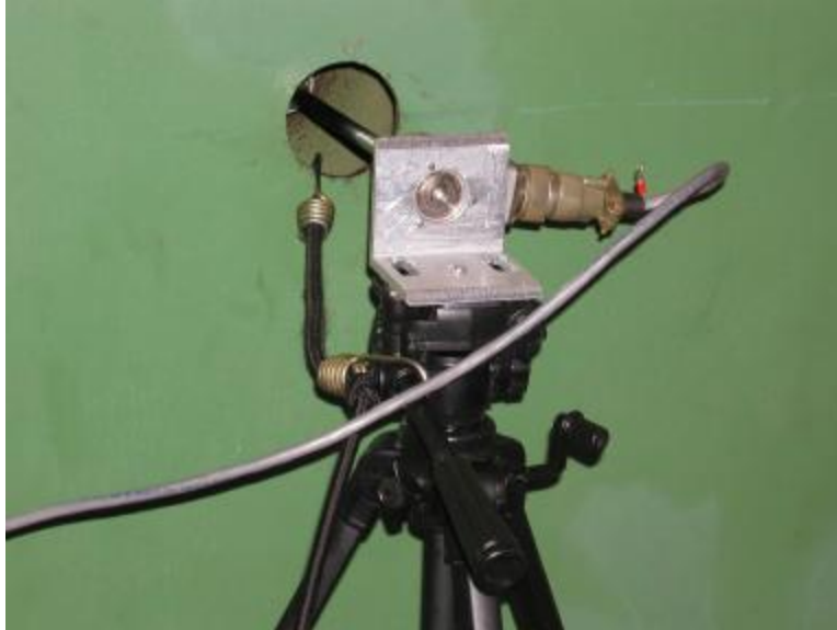
Figure 3-9. Detailed View of Encoder and Connection to Flywheel (GMW10; Williams Sour Lake Station; August 2003)
