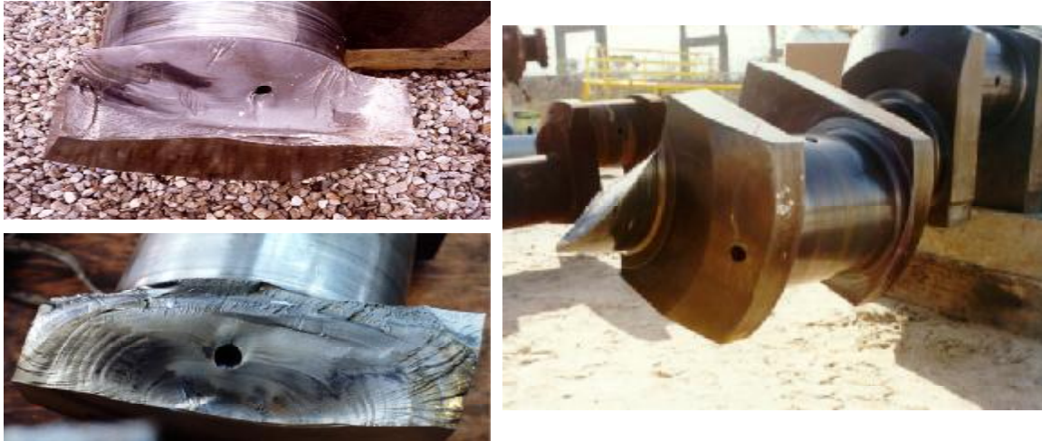
Figure 1-5. Integrity: Crankshaft Failure Examples – Need Methods of Avoidance
