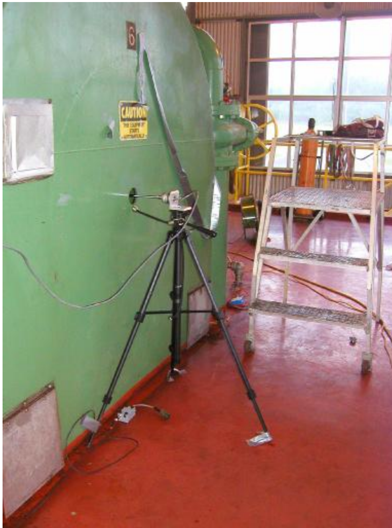
Figure 3-8. Encoder, Outboard of Flywheel on Mounting Tripod (GMW10; Williams Sour Lake Station; August 2003)
