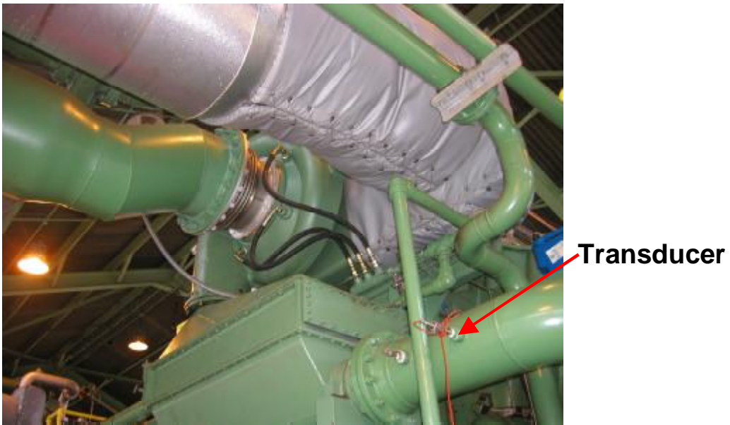
Figure 3. Turbocharger Added to GMW10 with High-Pressure Fuel Conversion, showing Air Manifold Dynamic Pressure Transducer
