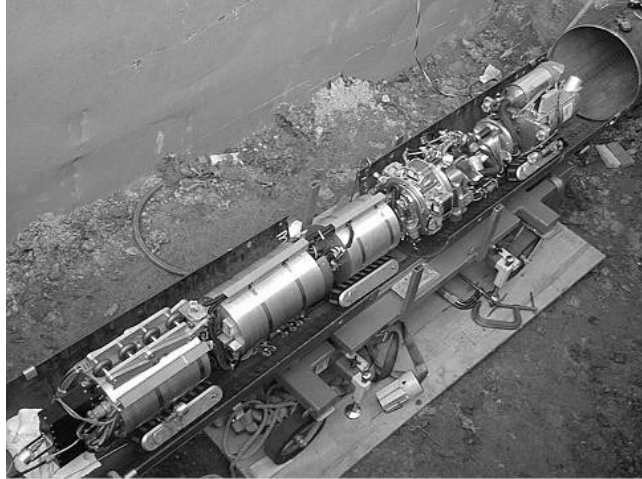
Figure 2 – Pacific Gas & Electric Internal Pipeline NDE System
