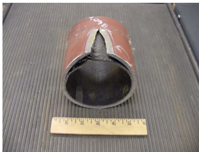
Figure 8 - Water-Jet Cut Section through Pipe Section with Liner
