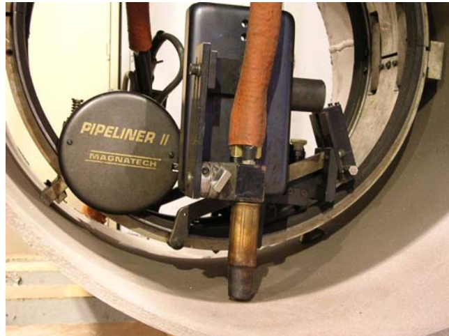
Figure 12 - Magnatech ID Welding Tractor Capable of Spiral and Ring Motion with Oscillation
