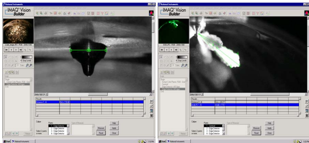
Figure 5 - Imaging software to quantify spray pattern
