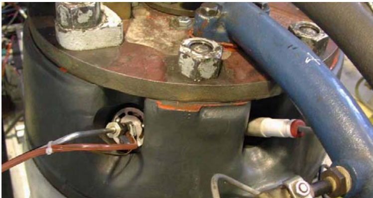
Figure 12 – GMV head with injector adapter (non-cooled)
