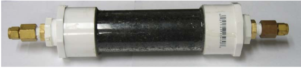
Figure 10: Sand pack for testing liquid-gas two-phase in porous media: effective length 12.7 cm, inner diameter 4.45 cm
