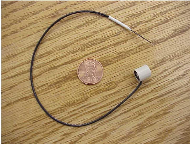
Figure 1. Acoustic transducer used in early development efforts
