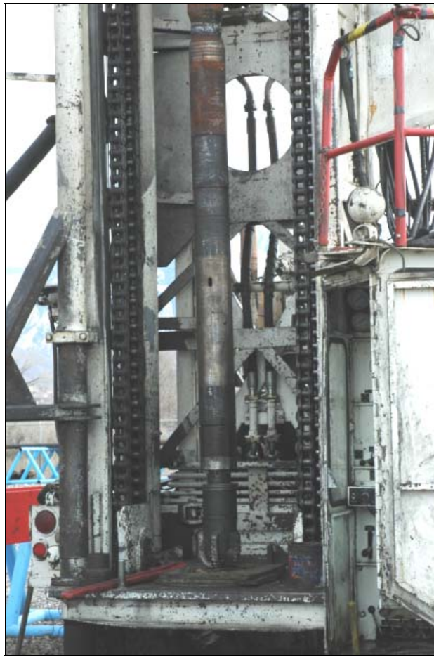
Figure 16. Hammer bit assembly ready for testing in a 100' well.
