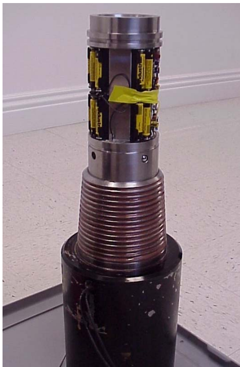
Figure 2. Electronic module supporting acoustic transducer
