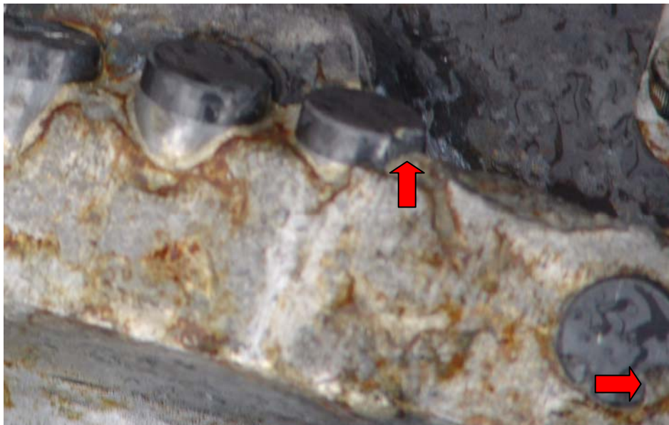
Figure 23. Damage to bit cutters after completing the 90' drilling test.
