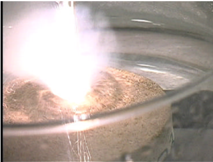
Figure 3-15 Water steam and waves created by laser beam.
