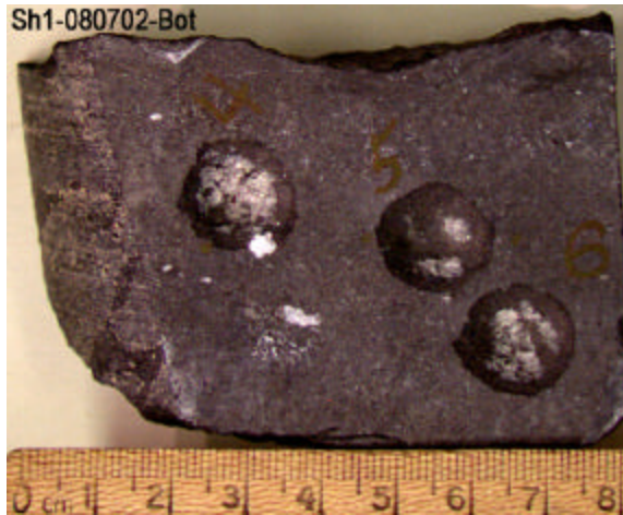
Figure 2-6. Shale sample Sh1, holes 4, 5 and 6. All holes were exposed to 3 bursts with one duration between bursts. Hole 5, with less visible melting, has an SE equal to the lowest in the test.
