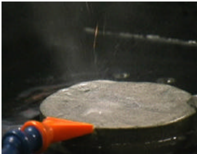
Figure 3-9 A 4 kW CO 2 laser beam only steamed the cross over water jet and did not reach the rock.
