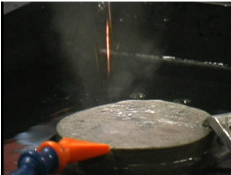
Figure 3-11 A 4 kW cw CO 2 laser beam interacted with a crossover water jet on a rock sample and created water vapor/steam. But it failed to reach the rock.
