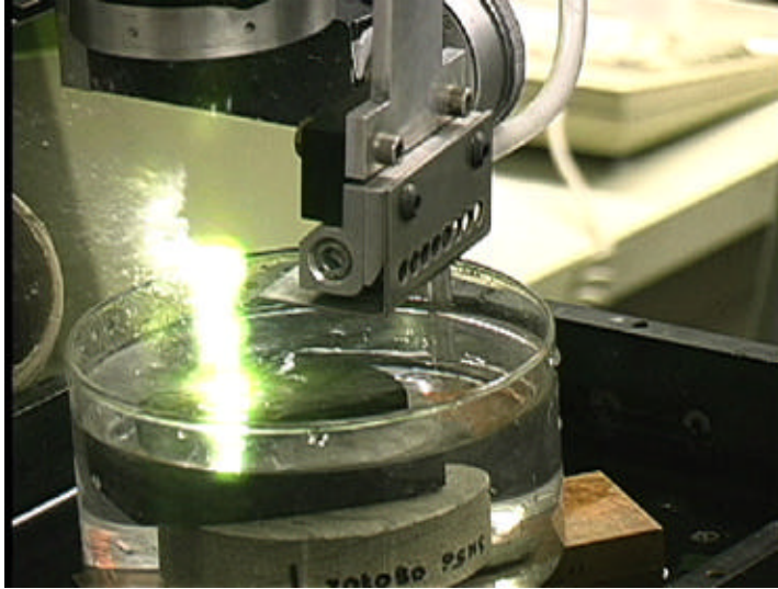
Figure 3-12 A 6.5 mm collimated Nd:YAG beam penetrated free water above rock and interacted with rock. A cross gas jet used is shown.
