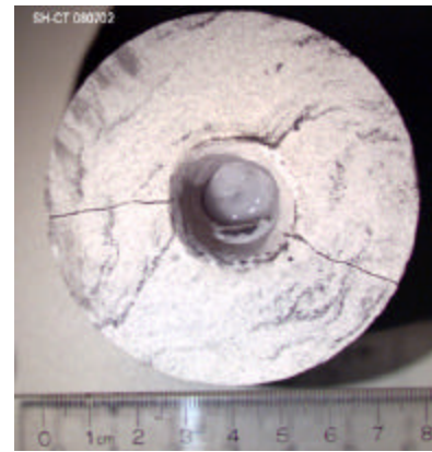
Figure 4-2 1 inch by 1.8 inch deep hole drilled by four bursts of 4 second duration 4 kw CO 2 laser beam on shale rock.
