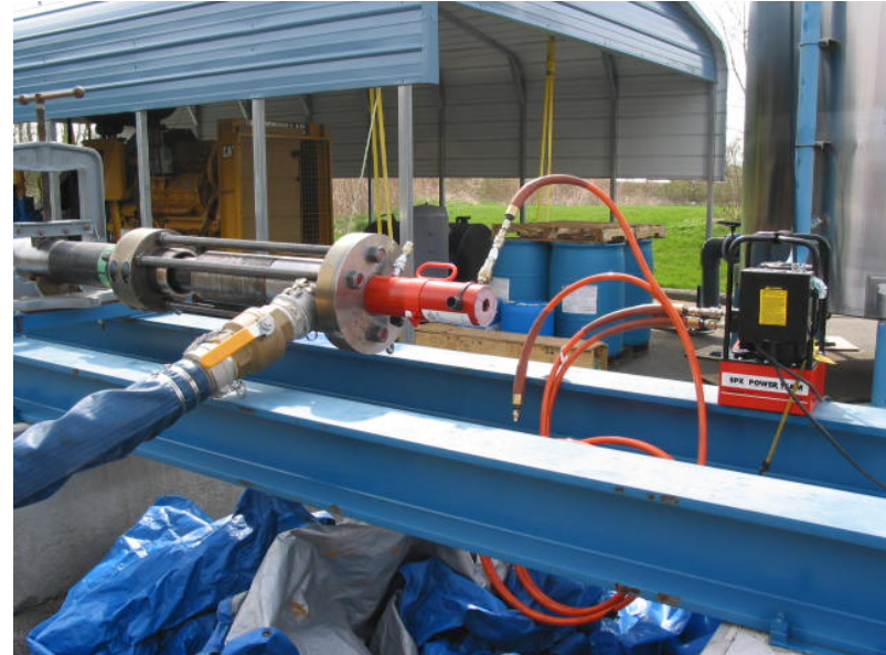
Figure 17: Field prototype valve assembly mounted in flow loop loading frame (left) with output monitors (right)
