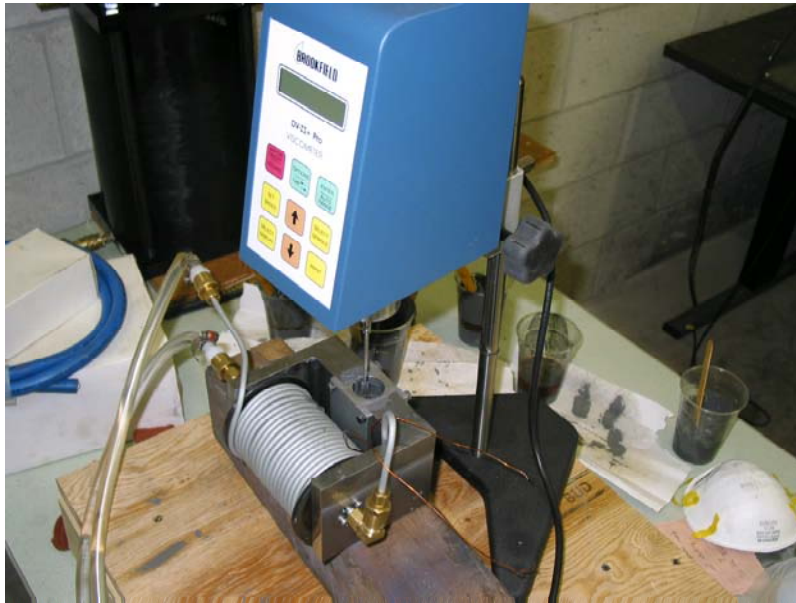
Figure 2: Photo of the viscometer test apparatus
