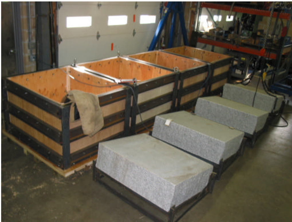
Figure 5: Granite blocks and concrete molds ready for assembly
