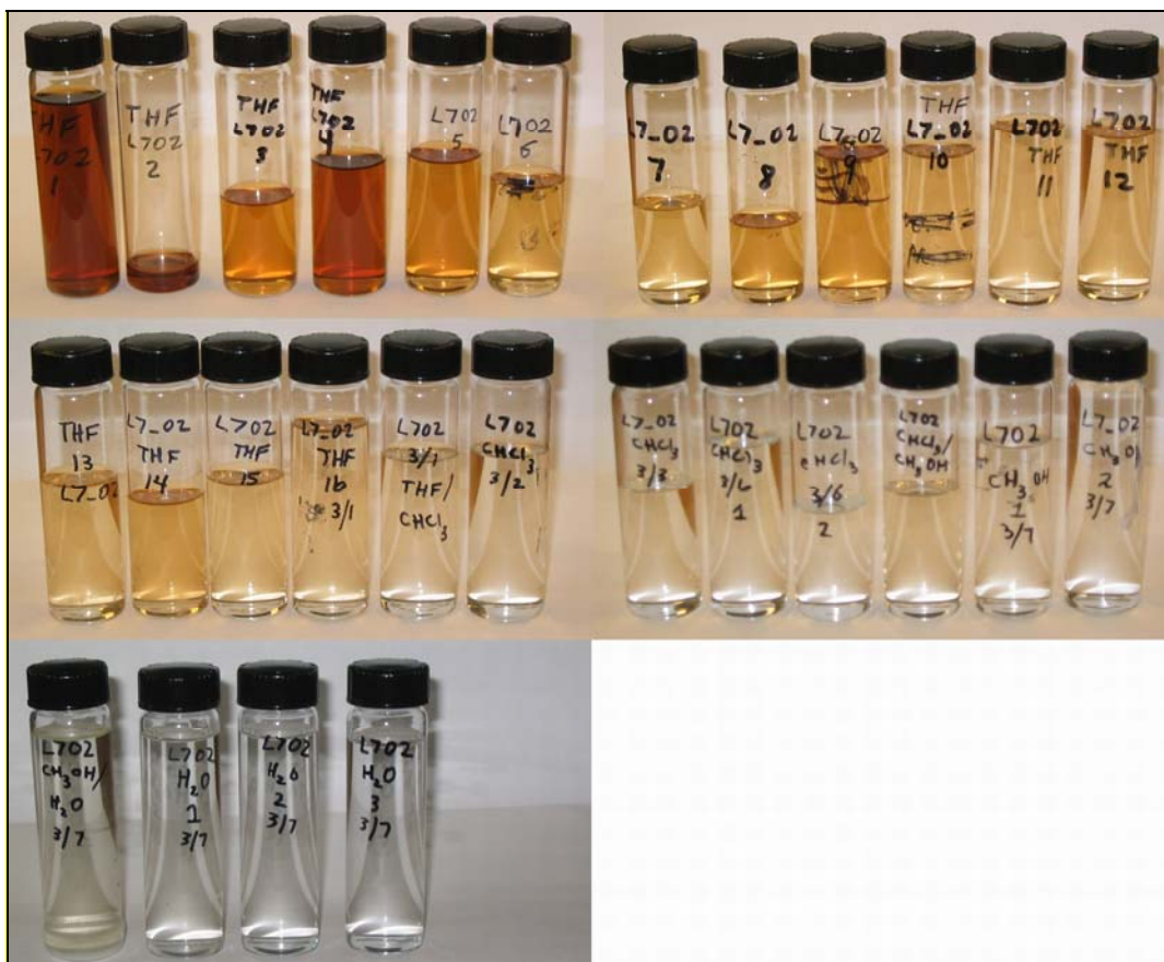
Plate 7 Effluents from cleaning L7_02. Solvents are tetrahydrofuran (THF), chloroform, methanol and water.
