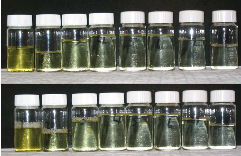
Plate 9 Effluent from core BF02 dodecane flood. Time increases from left to right. The lower image shows the same samples ~ 5 s after shaking to show the persistent foam associated with greater discoloration. The samples also exhibited appreciable UV absorbance (Figure 16)
