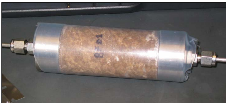
Plate 8 Core covered with Teflon® heat shrink material
