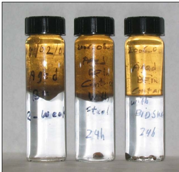
Plate 11 Two-phase (Soltrol 130/water) separation tests showing the effectiveness of surfactants in altering the wettability of crude oil-aged BF rock exposed to surfactant solutions for 24 h (left: No surfactant; center: STEOL CS-330; right: surfactin)
