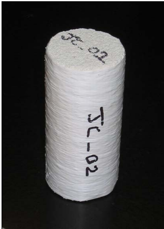
Plate 6 Core material: Joulters Cay oolitic outcrop wrapped in PTFE tape
