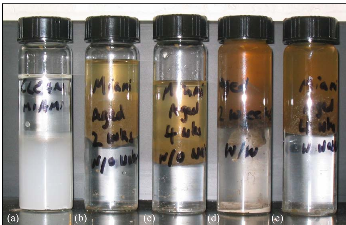
Plate 10 Crushed Miami oolite in RO water/Soltrol: (a) clean, (b) & (c) with no initial water saturation after 2 & 4 weeks under crude oil at 65 °C to show rapid change to oil wet state, (d) & (e) with initial water saturation after 2 & 4 weeks under crude oil at 65 °C to show slower progression through mixed-wet state.
