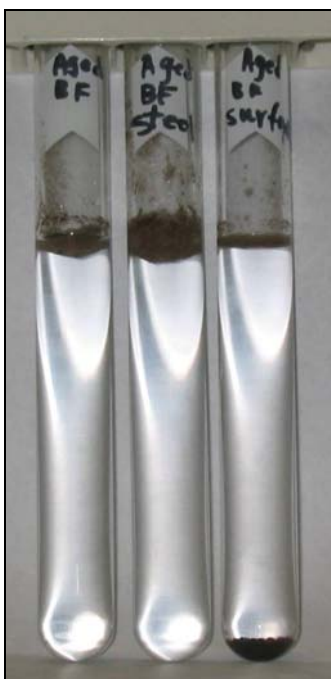
Plate 12 Water flotation tests showing the effectiveness of surfactants in altering the of crude oil-aged BF rock exposed to surfactant solutions for 24 h (left: No surfactant; center: STEOL CS-330; right: surfactin)
