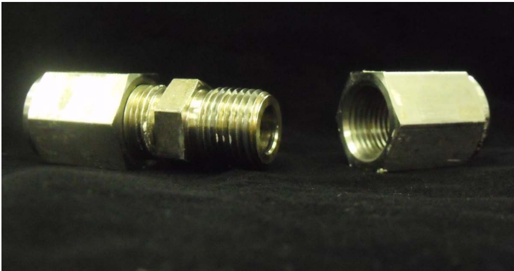
Figure 5. Device designed to act as a growth chamber that can be incubated in an oven at a Temperature of 115°C.
