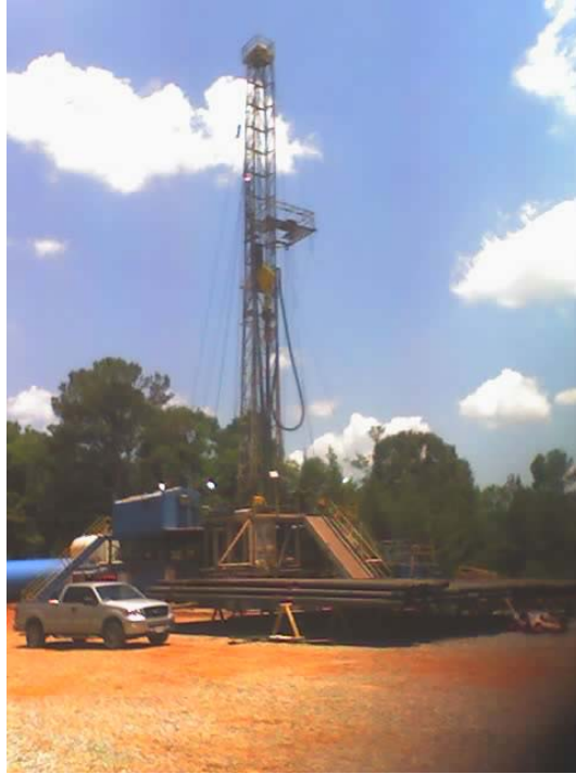
Figure 1. MSU geologists were on site in the summer of 2006 while approximately 400 ft of core were taken from this Eutaw Formation well near Laurel, MS. Fourteen samples of live core (approximately 8 in by 4 in) were acquired and placed in anaerobic storage at the drill site. Sample locations were based on electric log interpretation, drillers' reports, and visual inspection of the ends of the core.
