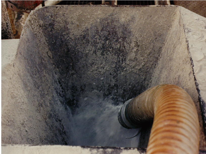
Figure 13. LWSA Additions to Mud at the Mud Hopper
