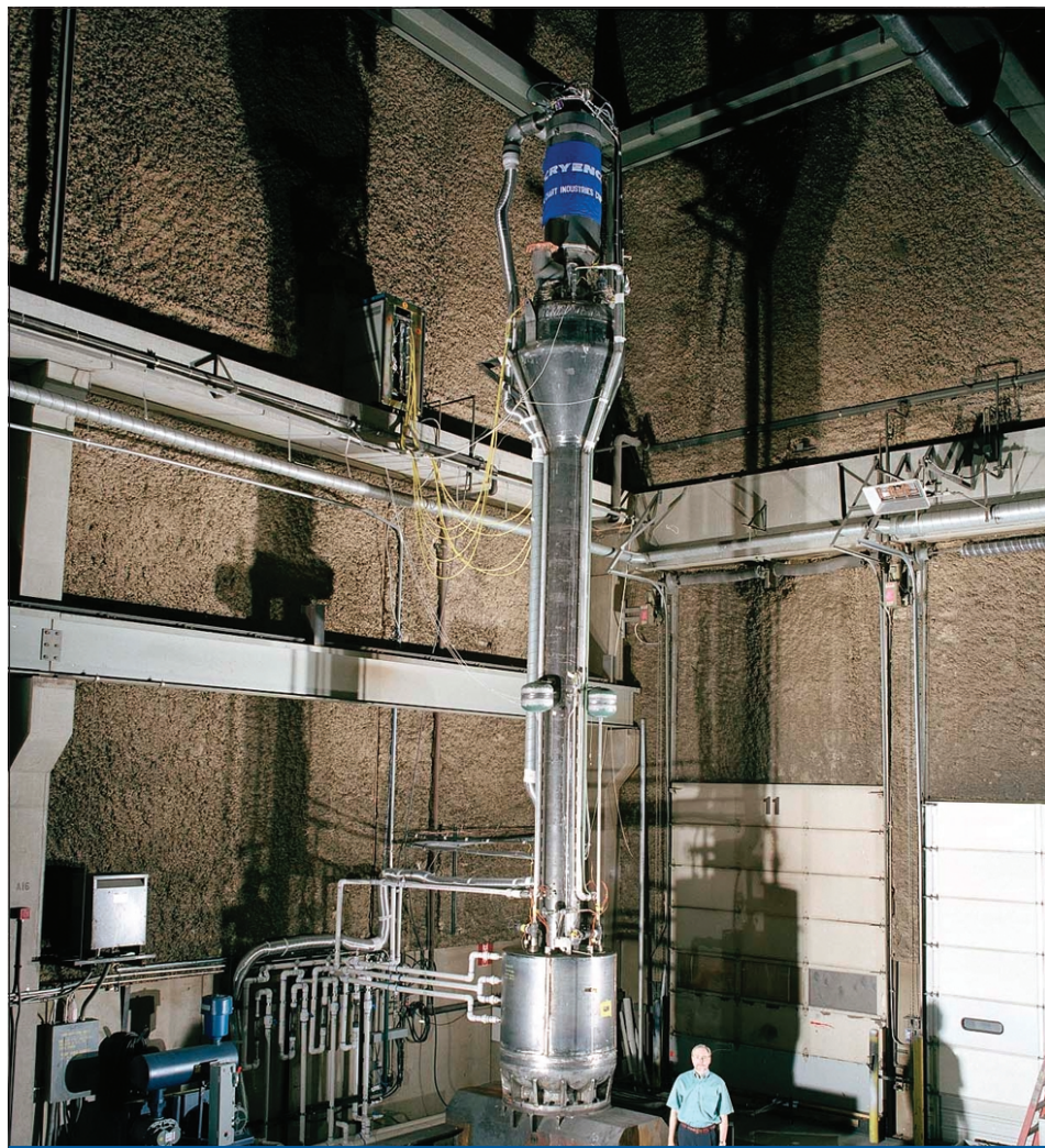
Figure 5: Current Prototype 500 GPD Acoustic Liquefier
