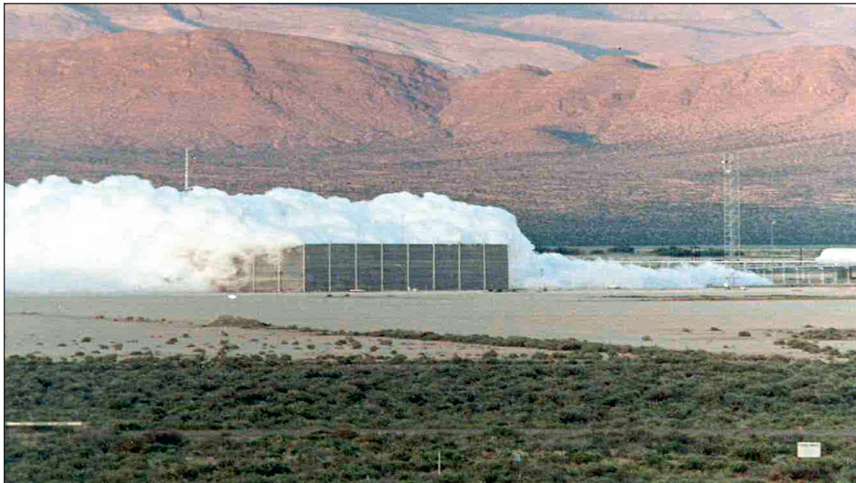
Figure 1: Field Test of Effect of Vapor Fence on LNG Vapor Cloud
