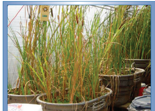
Figure 2. Pilot-scale constructed wetland treatment system for conducting experimental studies used to develop design parameters for building an onsite, demonstration-scale system.
