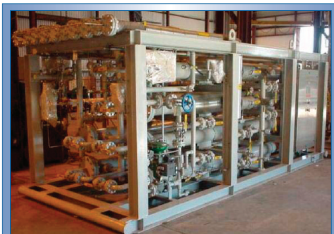
Figure 1. Skid-mounted nitrogen-rejection membrane separation unit destined for North Texas Exploration’s field site.
