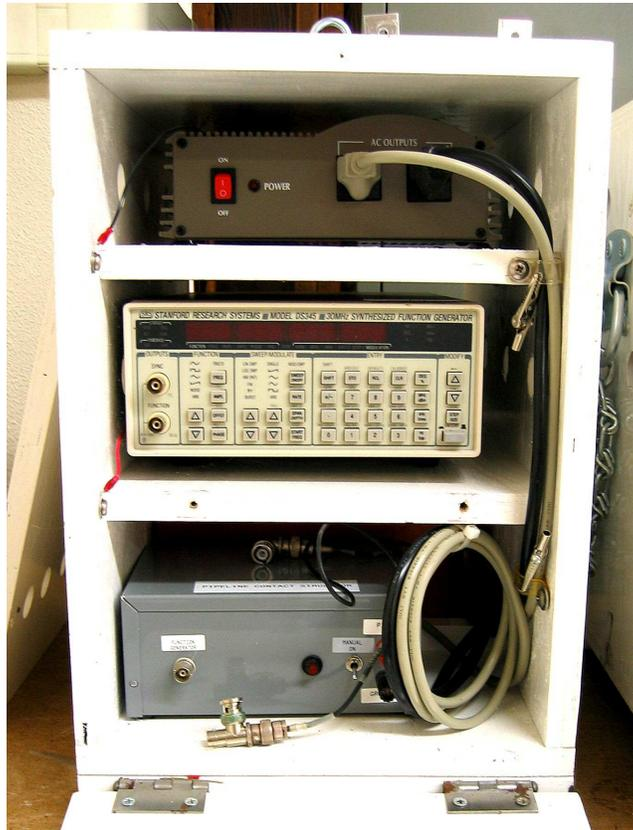
**Figure 22. Contact simulator configured for portable operation for field tests**
