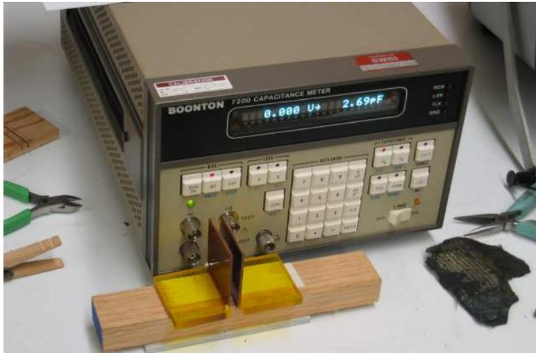
**Figure 8. Setup for measuring dielectric constant of pipe coating**
