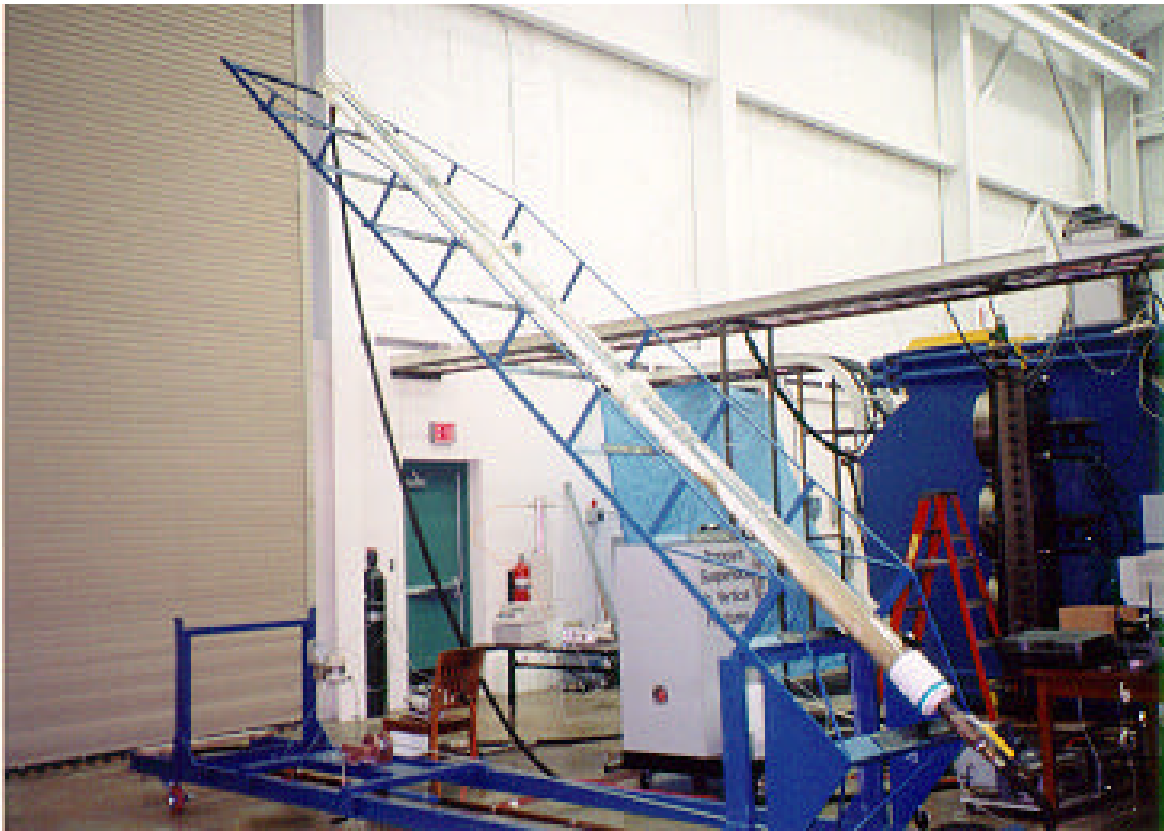
Fig. 3.6 Wellbore Simulator at a Deviated Angle of 45°
