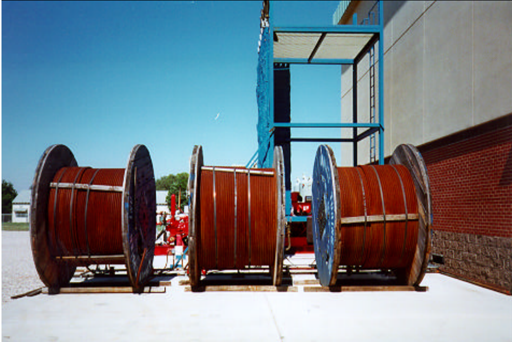
Fig. 3.1 Coiled Tubing System
