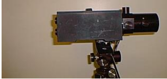
Figure 2. Photograph of the multi-spectral scanner mounted on a tripod.
