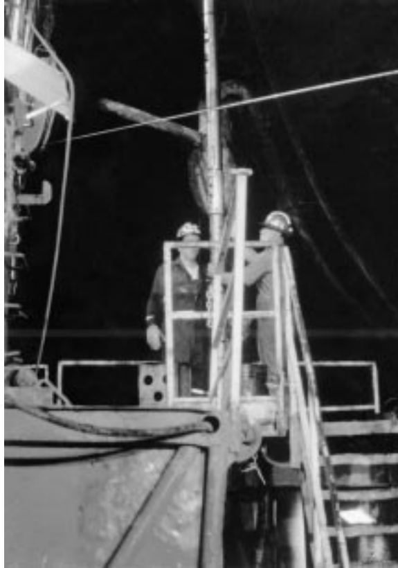
Figure 5. Schlumberger Sidewall CoreDriller ® tool tripping into the Atlas Lucas No. 1 well.
