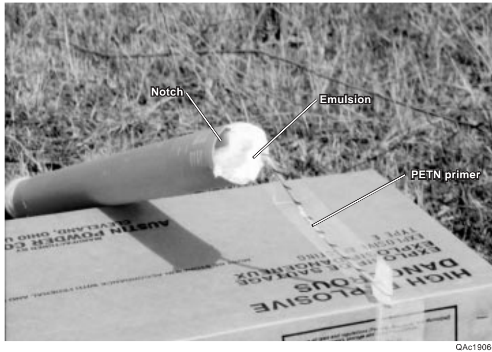
Figure 43. Low-velocity-emulsion shaped charge.
