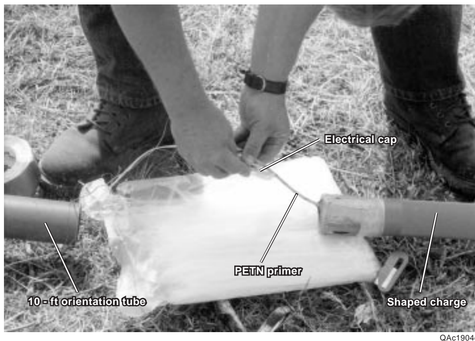
Figure 44. Low-velocity-emulsion shaped charge being prepared for detonation.
