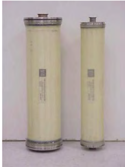
Figure 21. Comparison of 12-inch and 8-inch membrane modules. The 12-inch modules contain about 50 square meters of membrane, and the 8-inch modules contain about 20 square meters. The 12-inch elements made during this project were the first ones of that size manufactured by MTR. Their successful introduction will allow significant cost reductions on a per-square-meter-of-membrane basis for any membrane applications requiring high feed flow rates.
