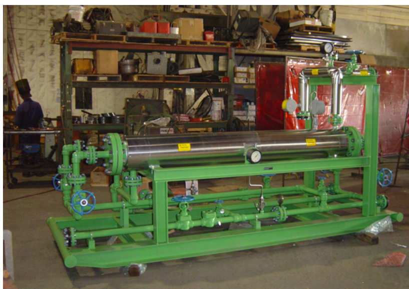
Figure 17. Photograph of a two-step membrane unit processing 0.4 MMscfd of natural gas to lower nitrogen content from 7% to 3.8% in Louisa, Kentucky. Operator is Twin Bottoms LLC. Interstate Energy operates a very similar system nearby.
