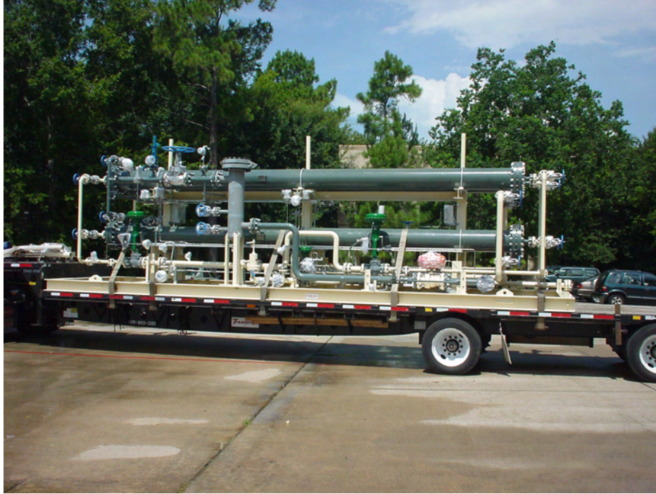
Figure 26. Commercial unit sold to Towne Exploration for treating gas containing 8-16% nitrogen.
