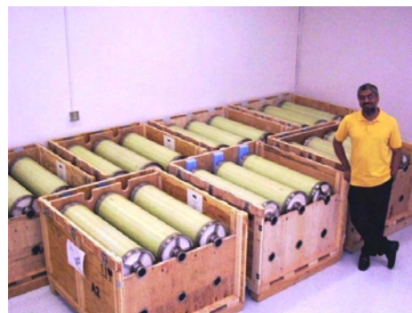
Figure 22. Ready-to-ship batch of MTR's new high-capacity 12-inch NitroSep™ modules.
