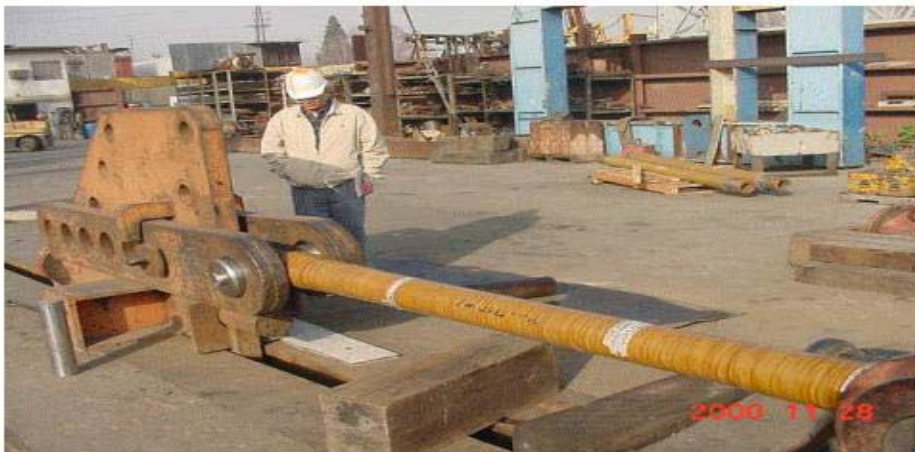
Figure 6: 10-Ft Full Diameter Tension Test
