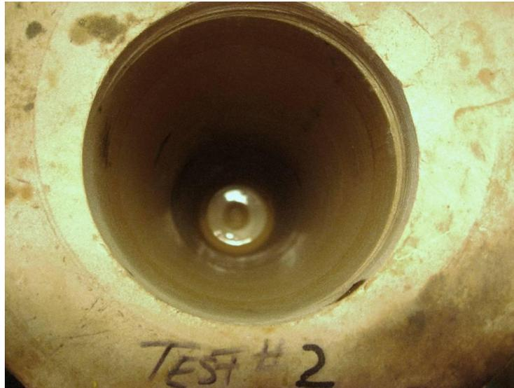
Figure 39: Test 2 Nearly Perfect Borehole
