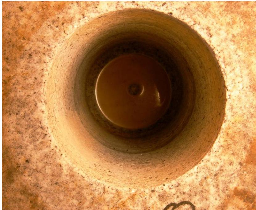
Figure 50: Test 11 Nearly Perfect Borehole
