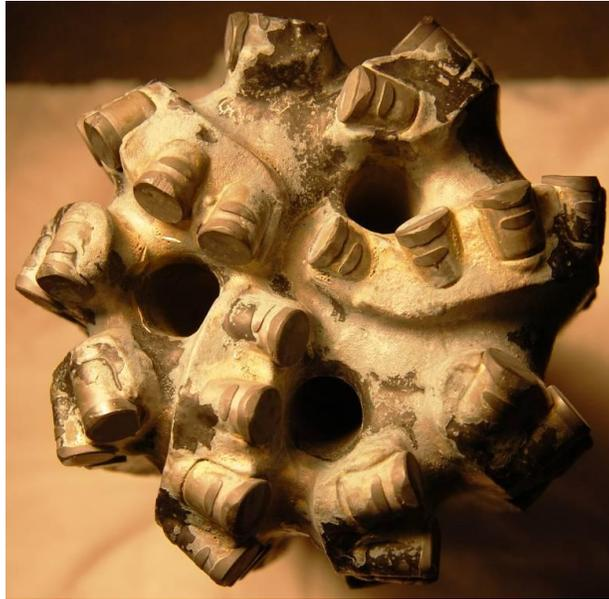
Figure 43: Test 4 Drill Bit After Test
