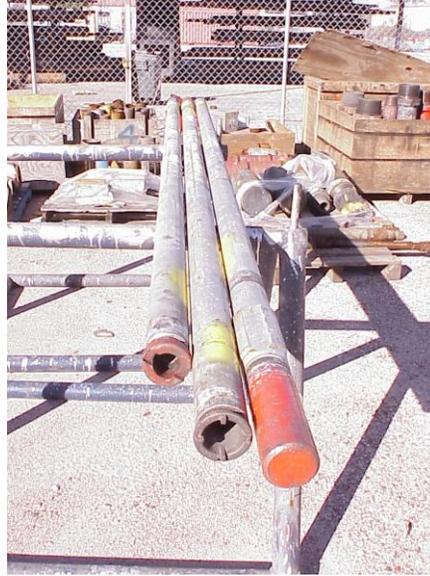
Figure 28: The Turbodrills for the Catoosa Test
