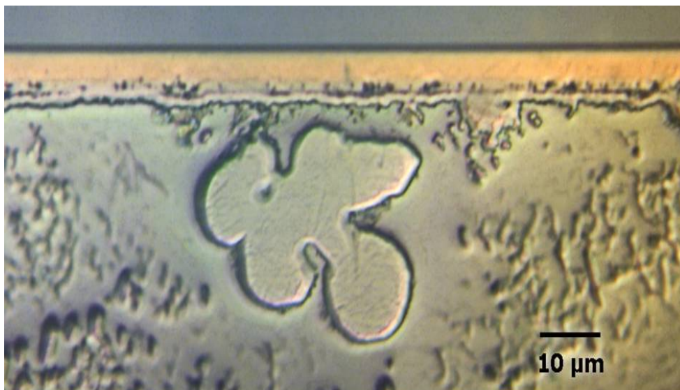
Figure 4.17. Optical image of reflowed Pb92.5-Sn5-Ag2.5 solder paste aged for 500 hrs at 250°C at 1000X.
