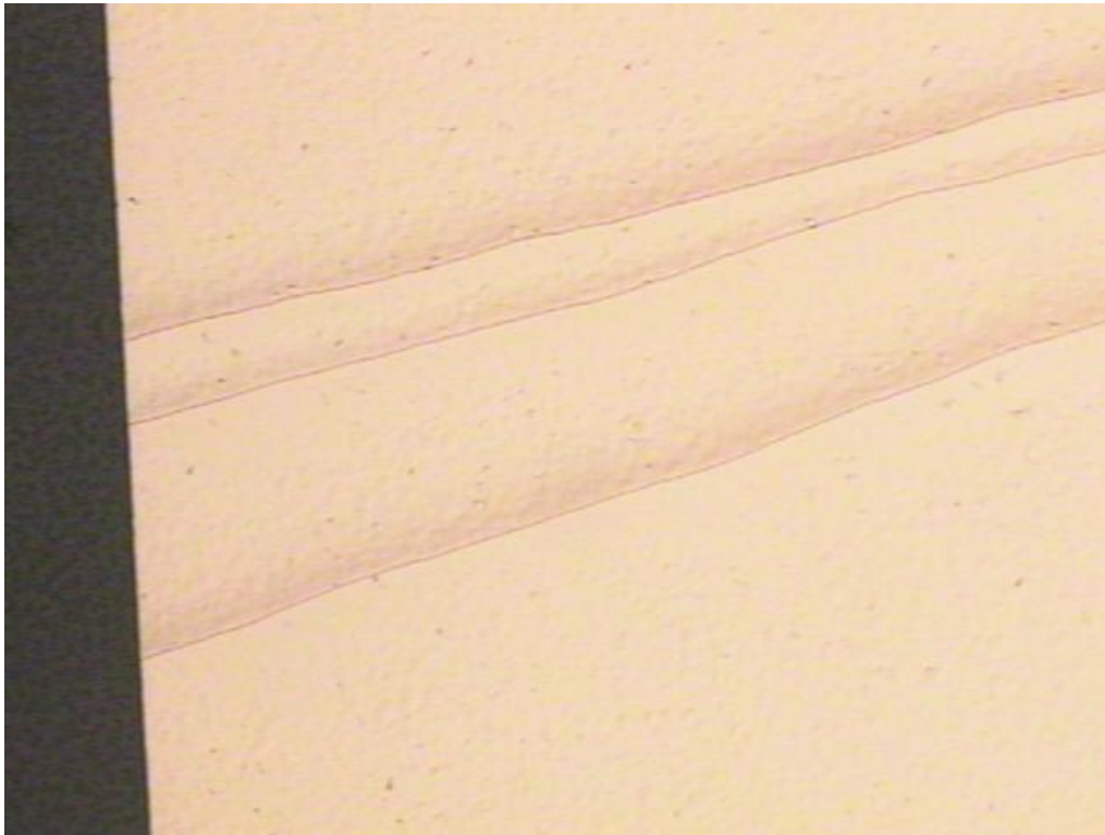
Figure 2.10. A microscope image of stress cracking on a 2000 A thick Cr sample.
