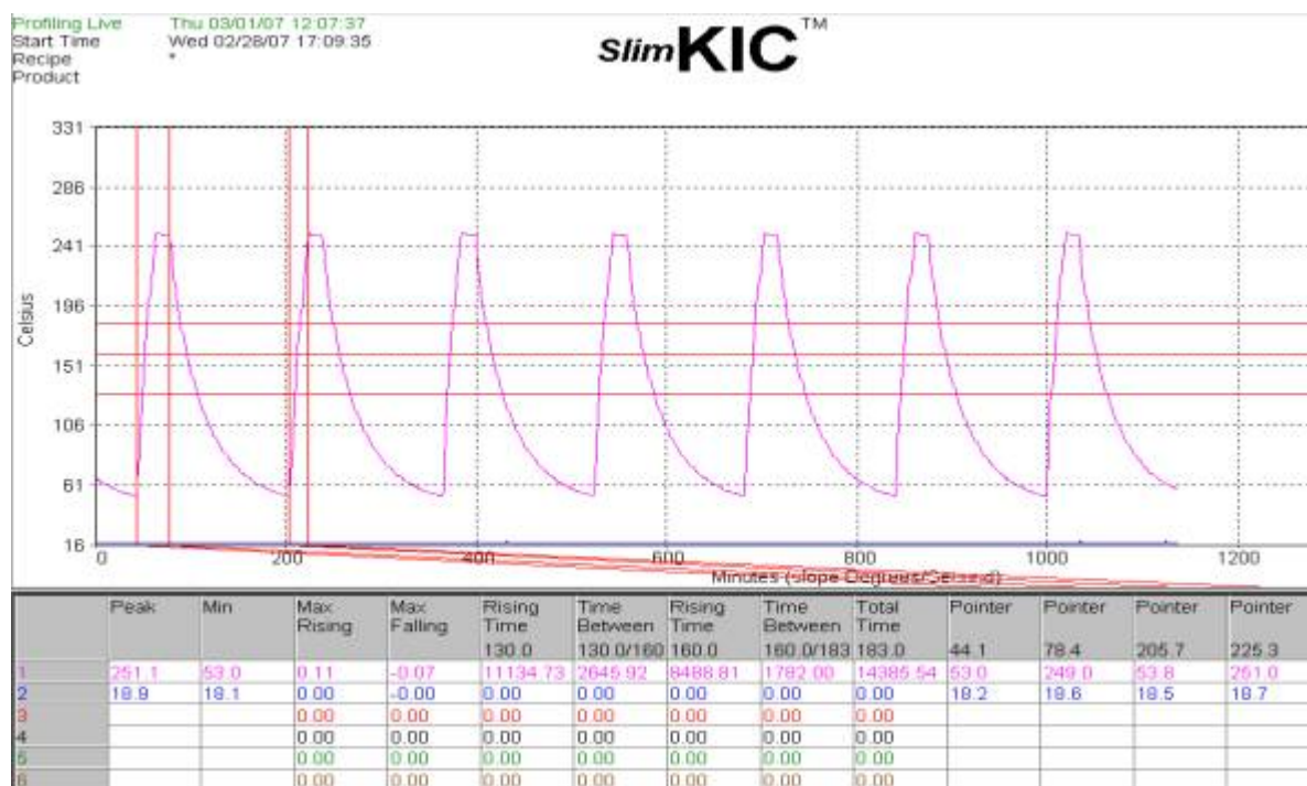
Figure 5.12. Temperature cycling profile (35 to 250°C).
