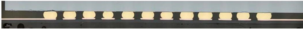
Figure 6.11. Failure in the die for coupons bonded at 175°C pick-up tool temperature.
