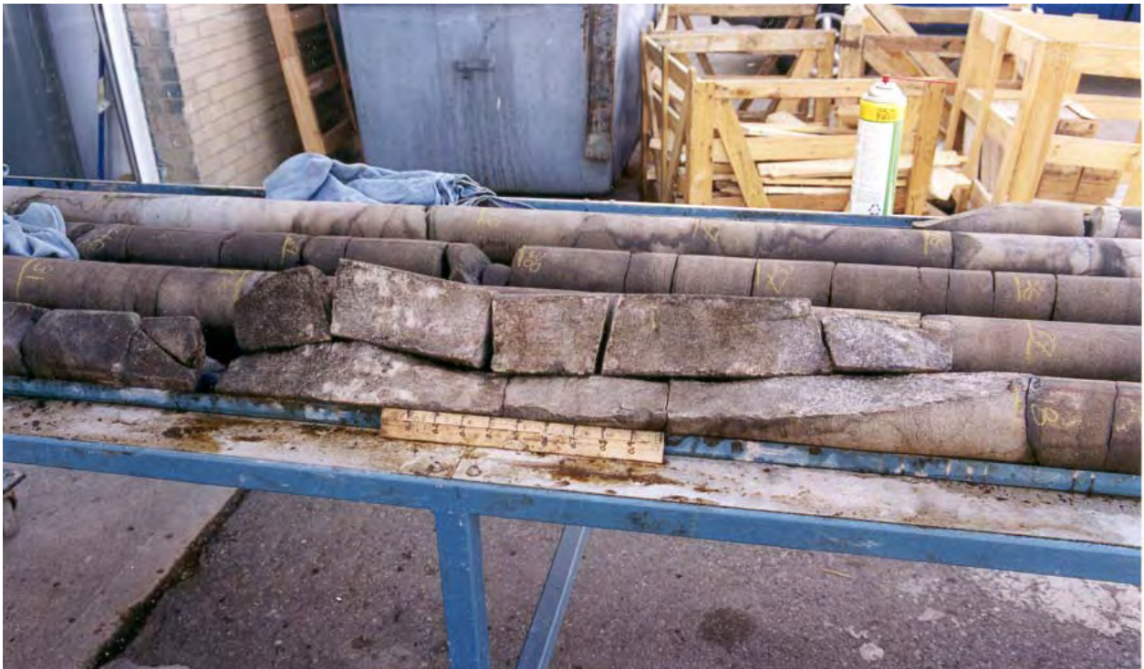
Disarticulated, bed bound natural fracture from Frontier Fm at 17,818 md in Barrett, Bullfrog #5-12. The fracture is lined with euheral carbonate crystals 2-3mm in size. Note non-planar geometry of the fracture face.
