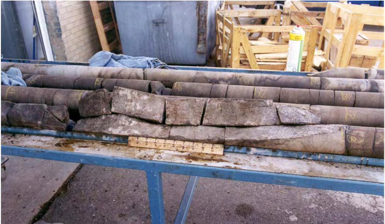
Disarticulated, bed bound natural fracture from Frontier Fm at 17,818 md in Barrett, Bullfrog #5-12. The fracture is lined with euhedral carbonate crystals 2-3mm in size. Note non-planar geometry of the fracture face.
