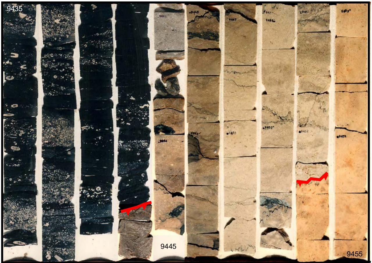
Figure 25. Core photos depicting cycle-top surfaces and facies picked by Saller and others (1999a, b) in the X1 well. Upper dark crinoidal unit corresponds to beginning of the Canyon Formation. Note that high thorium values on spectral gamma ray (fig. 24) correspond only to basal 2 ft of this unit. Interval considered a Stage 2 diagenetic event by Saller and others (1999a, b). Lowermost unit in figure marks beginning of upper Strawn reservoir interval. Judging from core porosity and permeability and wireline-log data, reservoir quality of this interval is good, with a maximum of 20 percent porosity and permeabilities slightly above 10 md. The porosity type found in the reservoir appears to be controlled by facies and grain type, as well as diagenetic alteration during exposure.
