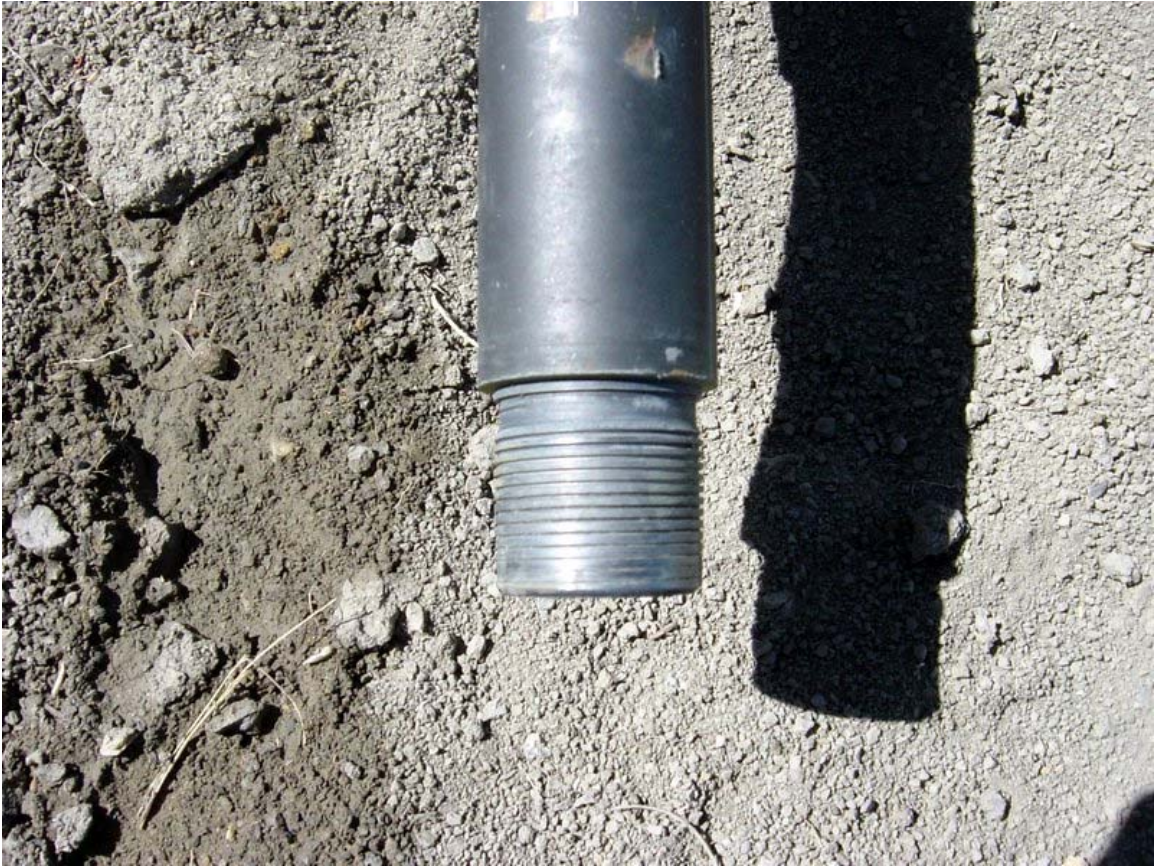
Figure A-5 – Worn Top Sub Connection After Backing Off
