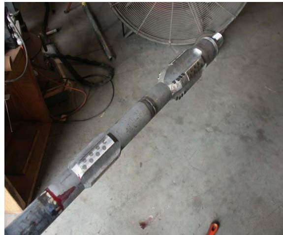
Figure 10- Reamer and Stabilizer
