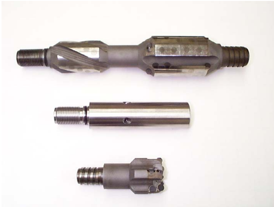
Reamer / stabilizer (top), Flow diverter (middle), Pilot bit (bottom)
