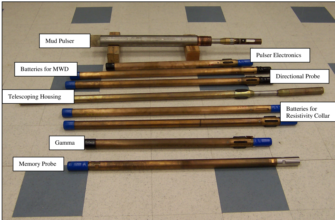
MWD, Gamma, and Memory Probes shown in Order of Assembly. Mud Pulser is on top, Memory Probe is on bottom.
