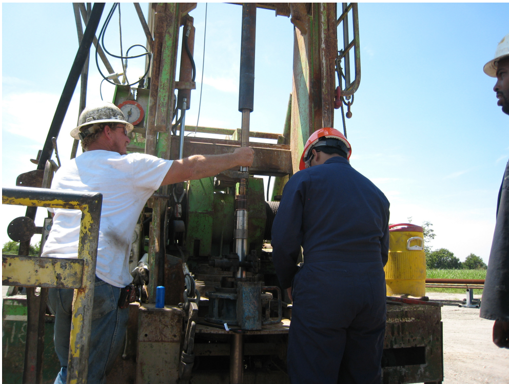
Making up BHA – 1 st Day of Test. Connecting Memory Probe to Top of Resistivity Collar
