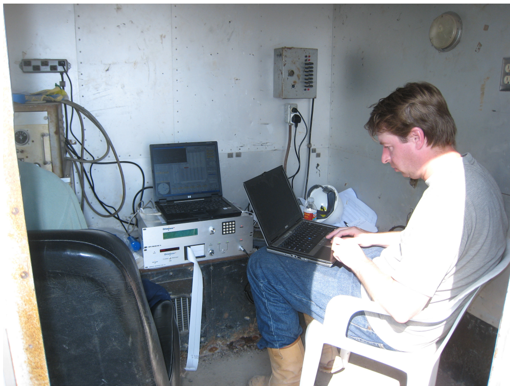
Surface System for Depth Tracking and Mud Pulse Decoding
