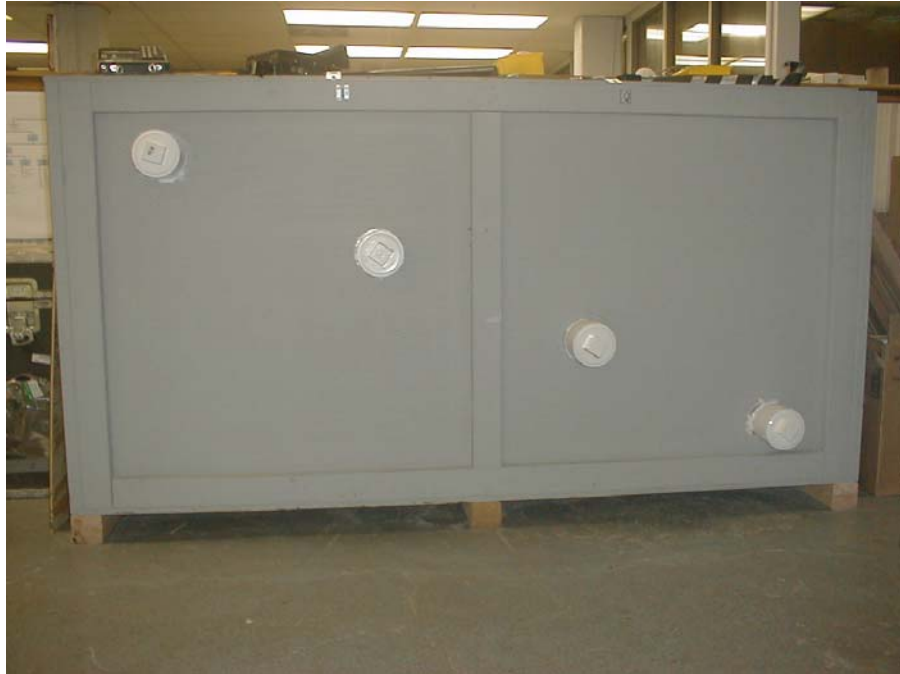
Figure 4-34. Stolar laboratory drill string radar borehole simulator.
