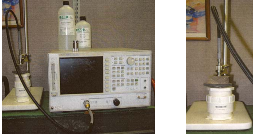
Figure 3-5. High-frequency instrumentation for measuring electrical properties of rocks.
