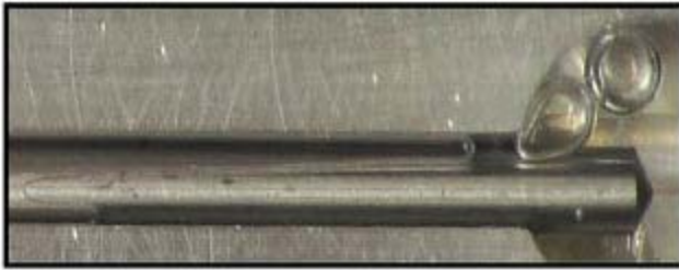
Figure 8.3-17. Counter-current imbibition. A bubble is emerging from the large tube. After snap-off, the meniscus invades the tube for some distance. However, much of this fluid comes from rearrangement of the arc menisci. Slot angle is 75^\circ and the gap is 0.17 mm.
