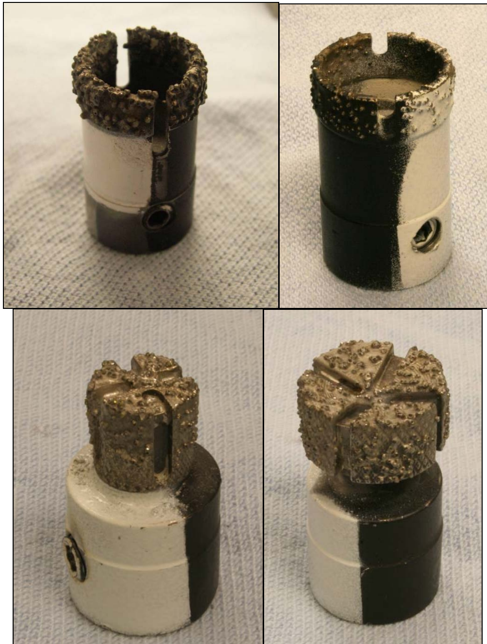
Figure 1. Core and full-faced drilling bits used for the high speed drilling tests. The core bit on the top left was used earlier in the program and the one on the top right was designed for consistency of diamond placement. Similar bits to the one on the top right were used in the final statistically designed and analyzed trials. Photographs of the small and large full-faced bits used are shown at the bottom of the figure.
