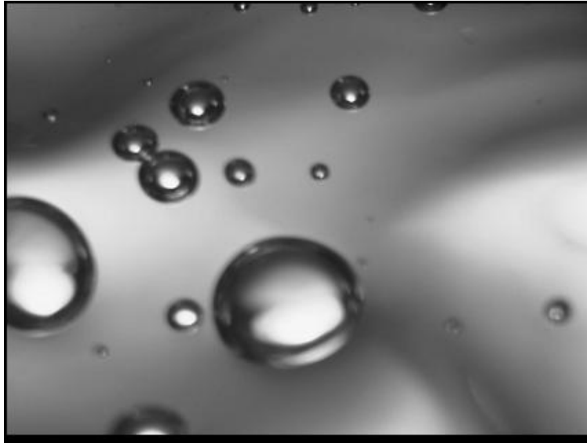
Figure 6. The Aphron Aggregate Breaks Up When Mild Swirling Force Is Applied
