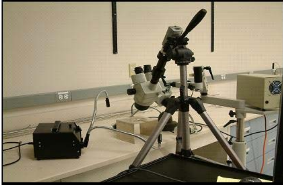
Figure 4. Set-Up for Microscope Slide Smear Test
