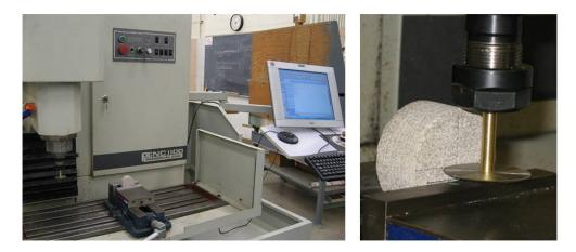
Figure 10-22. CCNBD specimen preparation
