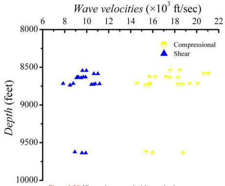
Figure 5-25. Ultrasonic wave velocities vs. depth
