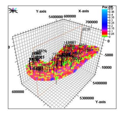
Figure 3-12. 3D model of the formation with north-south cross sectional cut
