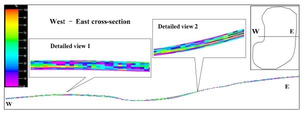
Figure 4-11: West-East cross-section view, 10 cm based RQD index
