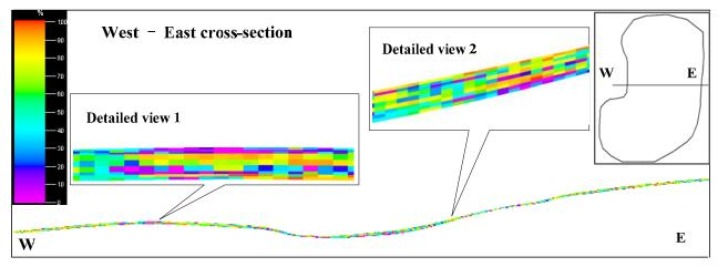
Figure 4-16. West-East cross-section view, 5cm based RQD index
