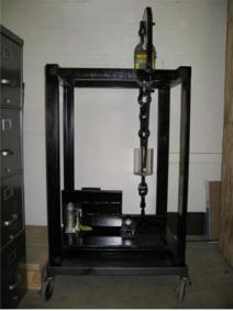
Figure 7-22. Tensile strength test apparatus
