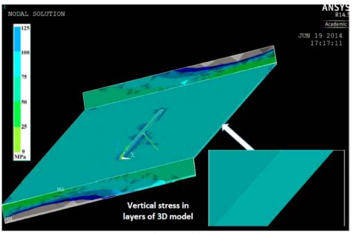
(b) 3D model Figure 5-29c. Contour map of vertical stress.
