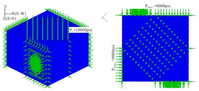
Figure 9-21. Boundary conditions for the Case 3, well axis is  $45^0$  to  $\sigma_{H}$ .
