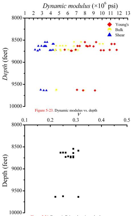
Figure 5-24. Dynamic Poisson's ratio vs depth
