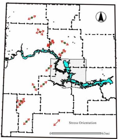
Figure 9-2. Orientations of maximum principal horizontal stress of the Bakken formation.
