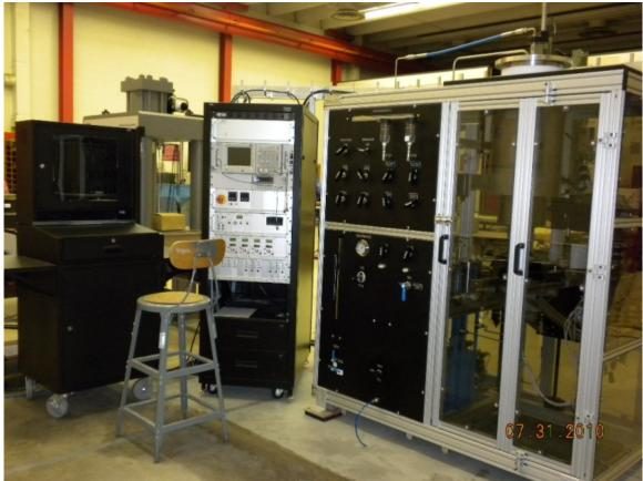
Figure 7-2 AutoLab 1500 used in this study.
