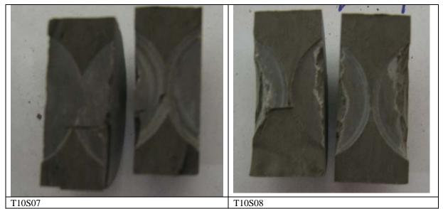
Figure 10-31. Fractured surfaces after tests for the test samples
