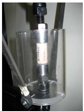
Figure 7-26. Tensile test apparatus (with both sides of the specimen was fixed)
