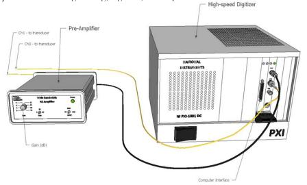
Figure 10-11. Setup of pre-amplifier and digitizer
