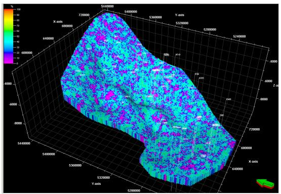
Figure 4-6. Populating RQD index in the 3D geological model in Petrel
