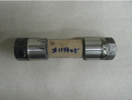
Figure 7-24. Specimen glued to steel caps
