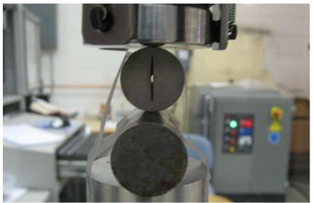
Figure 10-29. Shale sample under compression at MTS station
