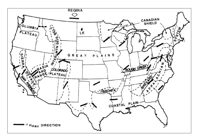
Figure 9-5 The maximum horizontal principal stress directions in continental United States based on the orientation of vertical hydrofractures (after Haimson, 1978; Narr and Burruss, 1984)
