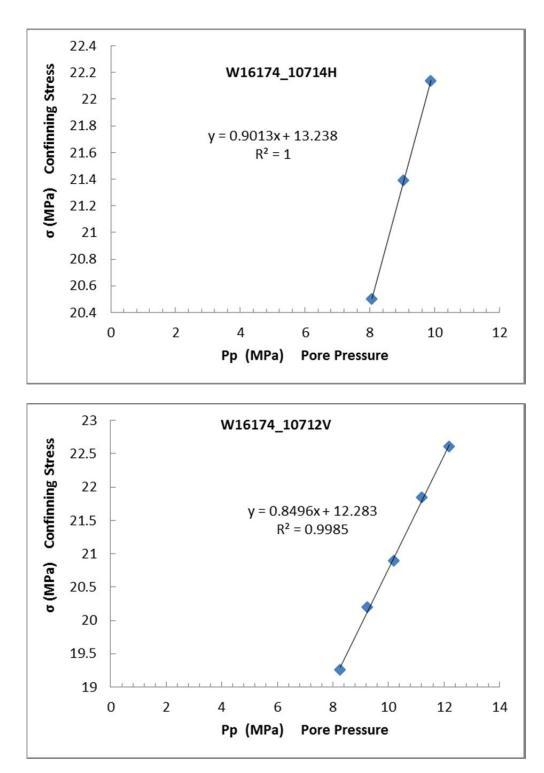
A.1.4 Static Moduli and Poisson's Ratio (Non-destructive)
