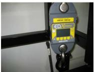
Figure 7-23. Dynamometer on top of tensile strength test apparatus
