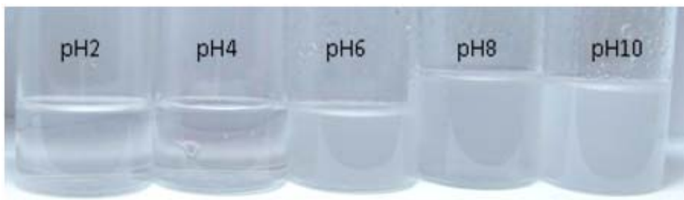
Figure 1-4: Sonication method for determining amine water solubility: 1 wt% THA water mixtures (pH2 -10) sonicated for 15 s.
