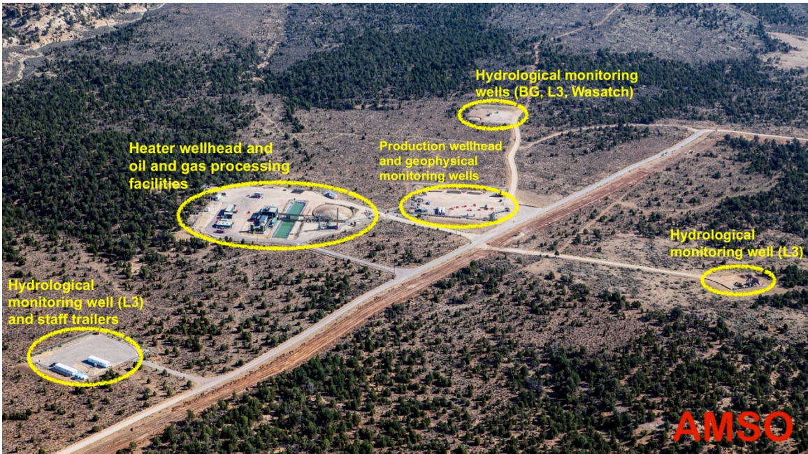
Figure 1. Aerial view of AMSO pilot test facility near Rifle, Colorado, with description of the site. Image provided by AMSO.
