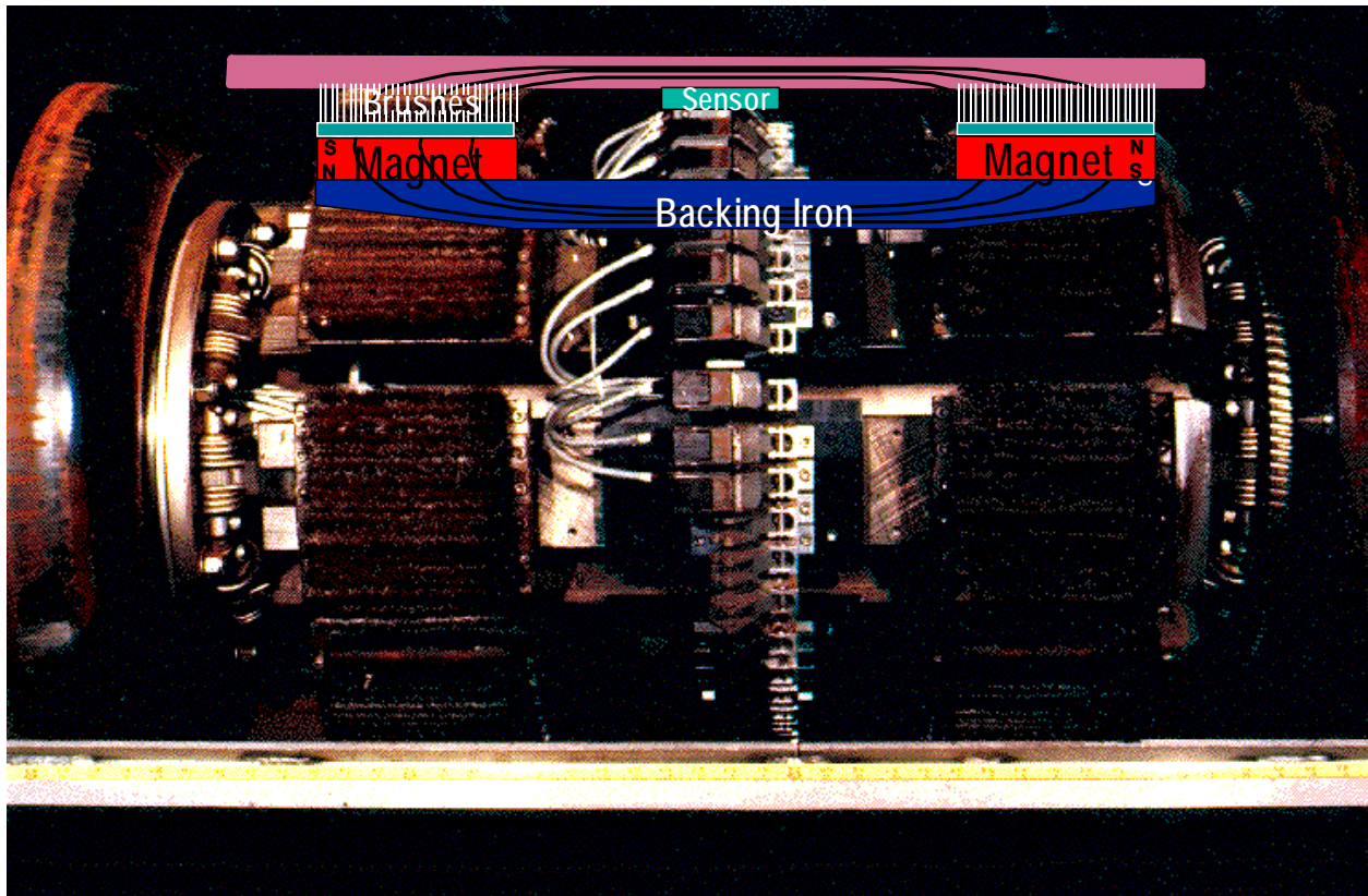
Figure 1. An axial MFL magnetizer.
