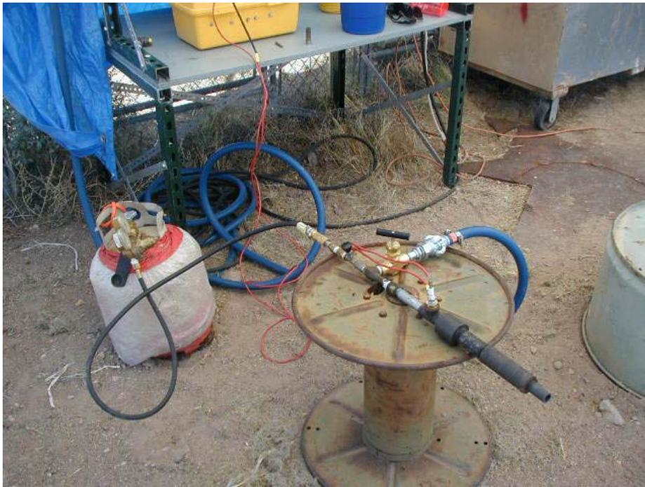
Figure 9. New Mexico Tech bench burner assembly.
