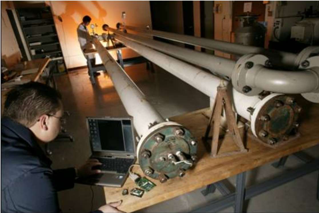
Figure 2-1. Non-line-of-sight pipeline wireless data transmission test setup.
